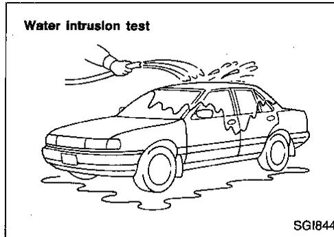
The incident may occur only during high humidity or in rainy/snowy weather. In such cases, the incident could be caused by water intrusion on an electrical part. This can be simulated by soaking the car or running it through a car wash.
