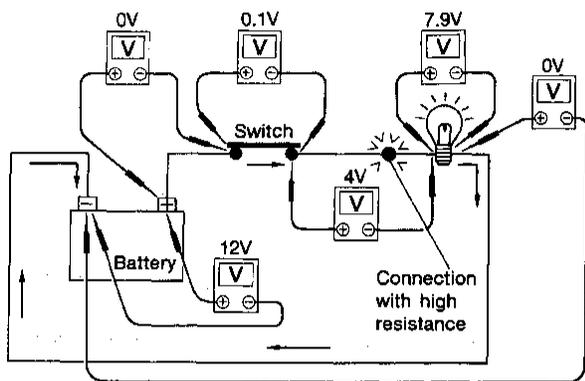
1. Connect the voltmeter as shown, starting at the battery and working your way around the circuit.
