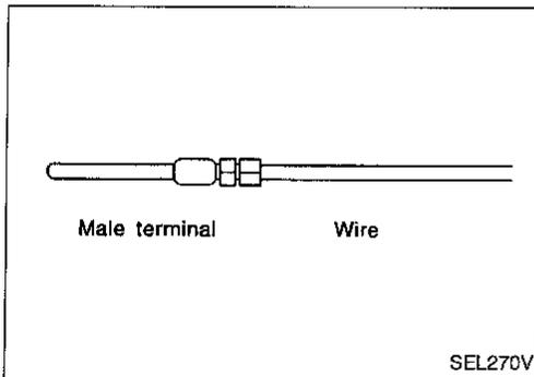
1. Assemble a male terminal and approx. 10 cm (3.9 in) of wire.
