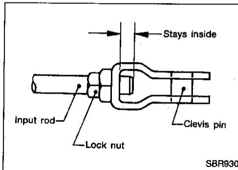
If necessary, adjust brake pedal free height.
