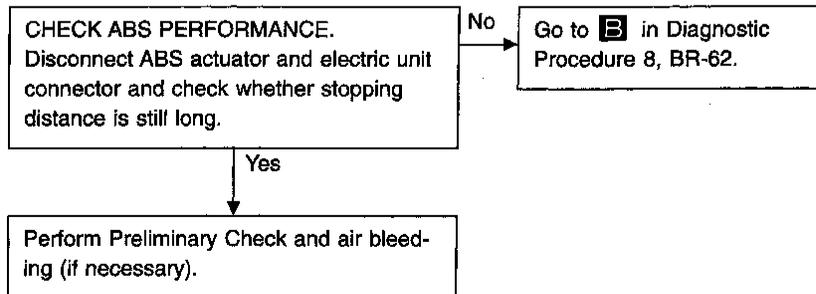
**Note:** Stopping distance may be longer for vehicles without ABS when road condition is slippery.
