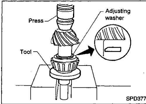
2. Select pinion bearing adjusting washer and drive pinion bearing spacer. Refer to "ADJUSTMENT", PD-24.
