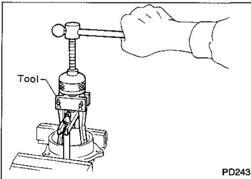
8. Loosen drive pinion nut.
