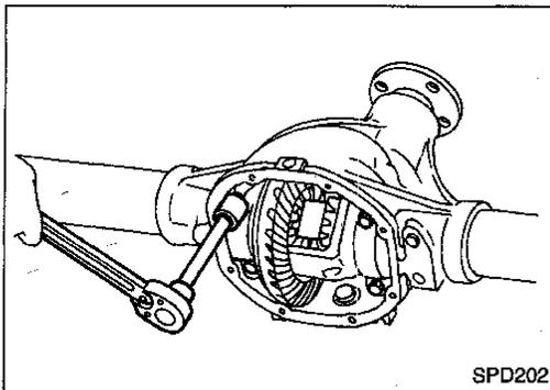
4. Remove differential case assembly with pry bar.
