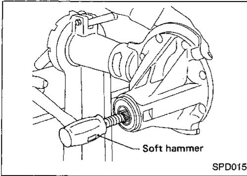
7. Remove drive pinion with soft hammer.
