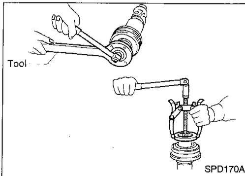
3. Remove locking nut using Tool.
