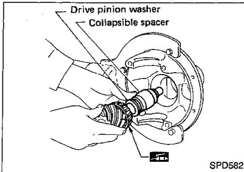
7. Install companion flange and hold it firmly. Insert pinion into companion flange by tapping its head with a soft hammer.
