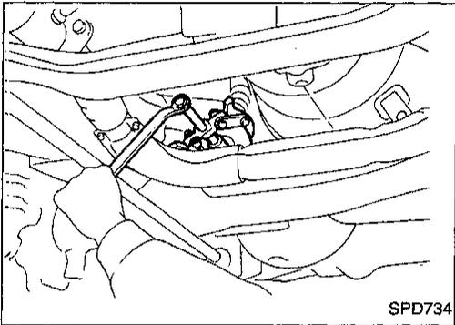
3. Remove companion flange using puller.
