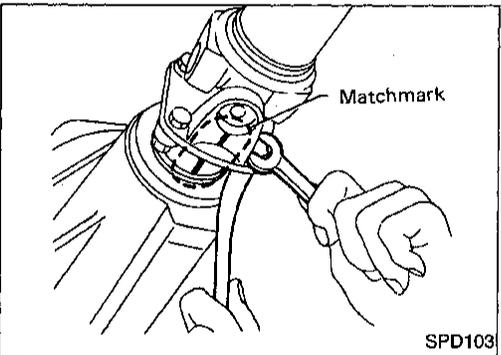
2. Remove propeller shaft.
