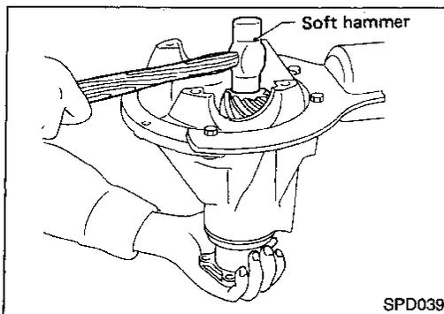
8. Temporarily tighten pinion nut until there is no axial play. The threaded portion of drive pinion and pinion nut should be free from oil or grease.
