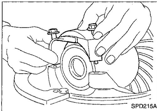
5. Install carrier and bearings into the final drive housing. Install side bearing caps. Torque the bolts and tap on the caps with a soft hammer to seat the bearings.
