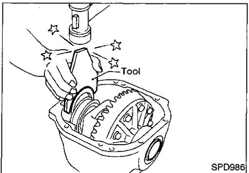
4. Use Tool to place original carrier side bearing preload shims on the carrier end, opposite the ring gear.
