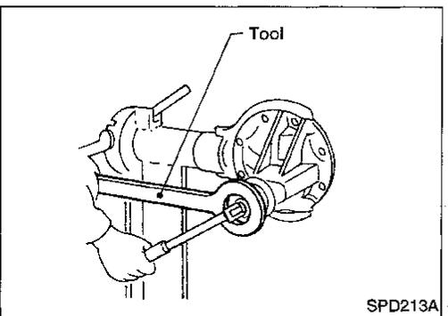
5. Remove drive pinion nut with Tool.
