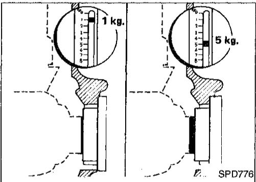
7. If necessary, correct the carrier bearing preload by adding to or subtracting from the total amount of shim thickness. Add shim thickness to increase turning force on the carrier. Subtract shim thickness to decrease turning force on the carrier.
