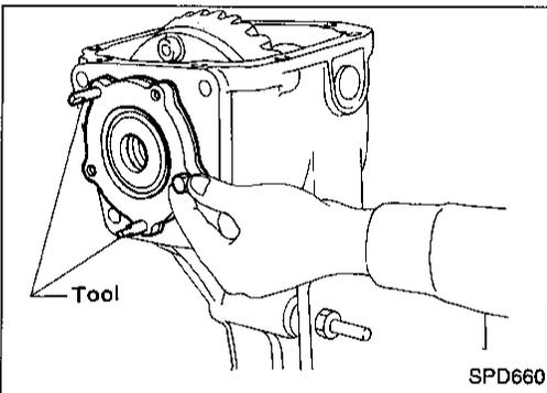
12. Install side oil seal to side retainer.
