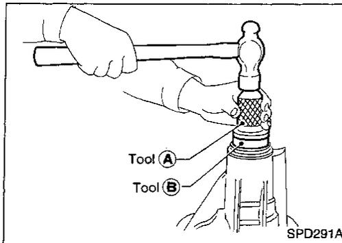
6. Install drive pinion washer, collapsible spacer and drive pinion in gear carrier.
