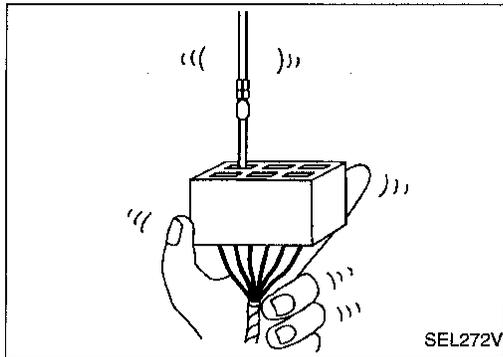
4. While moving the connector, check whether the male terminal can be easily inserted or not.
