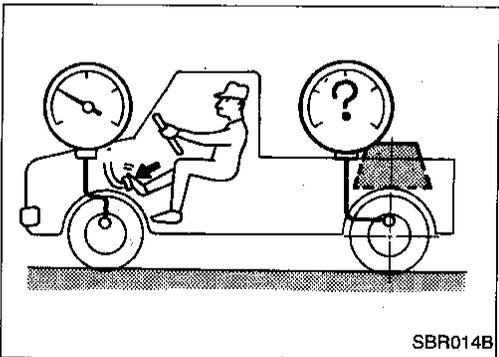
7. Set down weight slowly over axle center so that sensor spring length becomes the same as when in loaded condition (refer to table below). Check rear brake pressure in the same way described in step 6.
