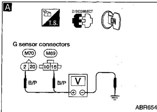
**CHECK G SENSOR POWER SUPPLY CIRCUIT.**
