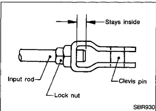
If necessary, adjust brake pedal free height.
