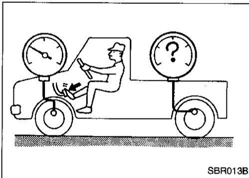
4. Install pressure gauge to front and rear brake air bleeder.
