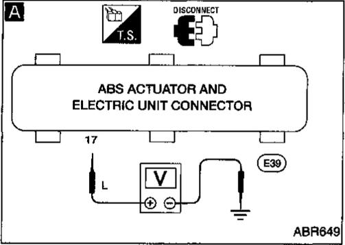
Diagnostic Procedure 3 (Motor relay or motor)
