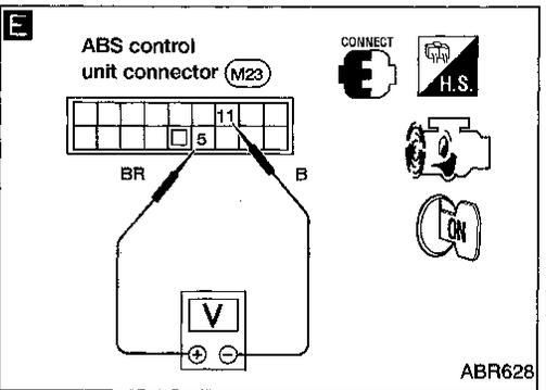
**Main Power Supply and Ground Circuit Check**
