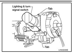
Remove the screws, release the clip, and remove the spiral cable.
