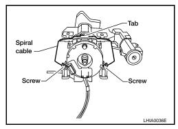
6. Remove the spiral cable connectors.
