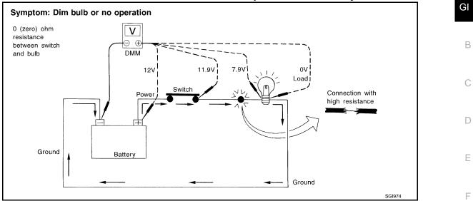
Measuring Voltage Drop — Steb-by-Step
