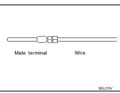
3. While holding the wire of the male terminal, try to insert the male terminal into the female terminal. CAUTION:
