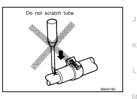
To reinstall the rubber hose securely, make sure that hose insertion length and orientation is correct. (If tube is equipped with hose stopper, insert rubber hose into tube until it butts up against hose stopper.)
