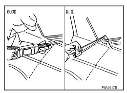
When welding HSS panels, use spot welding whenever possible in order to minimize weakening surrounding areas due to heat.
