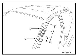
Determine cutting position and record distance from the locating indent. Use this distance when cutting the service part. Cut outer front pillar over 60 mm above inner front pillar cut position.
