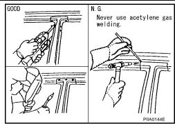
The spot weld on HSS panels is harder than that of an ordinary steel panel.
