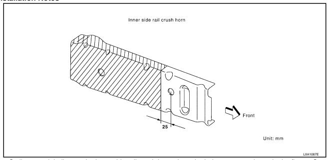
Scribe a straight line on the inner side rail crush horn along the hole center as shown in the figure. Cut off inner side rail crush horn along scribed line.
