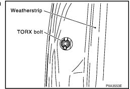
4. While pulling the outside handle, remove the door key cylinder assembly or escutcheon.
