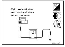
4. Check continuity between power window and door lock/unlock switch RH connector D105 terminal 11 and ground
