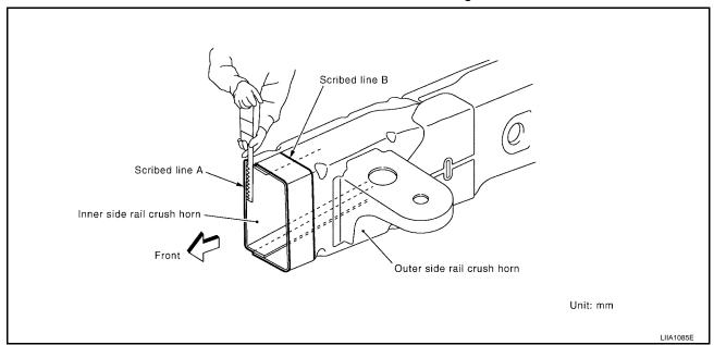
• Cut inner side rail crush horn at 45 mm backward cut position of cut line A. (along line B)
