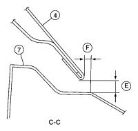
1. Hood hinge 2. Hood stay 3 4. Hood assembly 5. Front grille 6. 7. Front fender A. 8.0 mm (0.315 in) B. C. 0.8 mm (0.031 in) 8.0mm (0.315 in) D. 0.0 mm (0.00 in)
