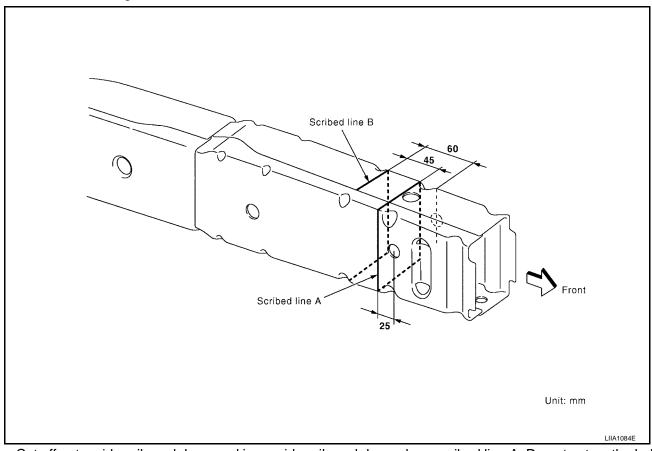
• Cut off outer side rail crush horn and inner side rail crush horn along scribed line A. Do not cut on the hole.
