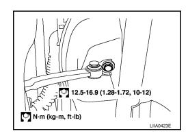
5. Remove the door-side hinge nuts and bolts, and remove the door assembly.
