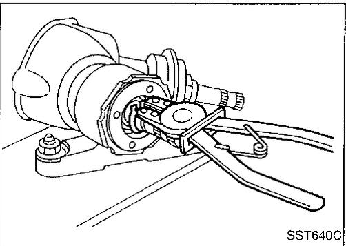
20. Install snap ring in the groove correctly.
