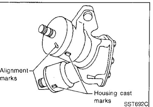
26. Locate position of highest torque.
