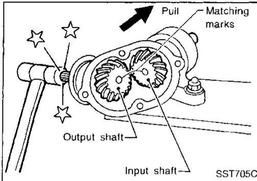
7. Remove rear cover with Tool (pin-type lock nut wrench). Remove thread locker residue from the transfer gear housing using a toothbrush and thinner.
