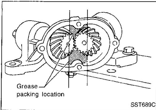
22. Pack input and output shaft gears with grease.
