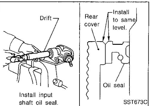
21. Apply grease to input and output seal lips. Install oil seals with drift.
