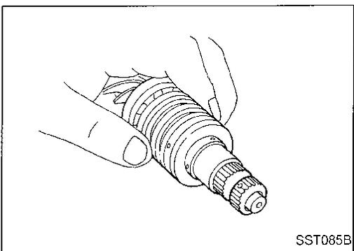
10. Install new pinion seal ring (made of Teflon) on pinion gear assembly.
