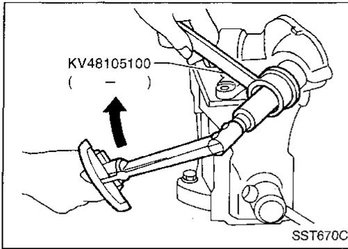
11. While holding inner nut using Tool, tighten lock nut using a torque wrench.
