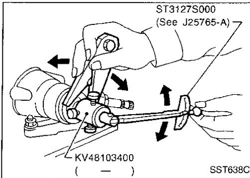
17. While adjusting rear cover, measure rotating torque of input and output shaft (as a unit) with Tools.
