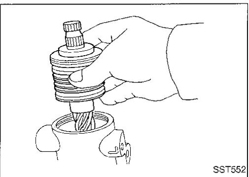
12. Install pinion assembly to rear housing.
