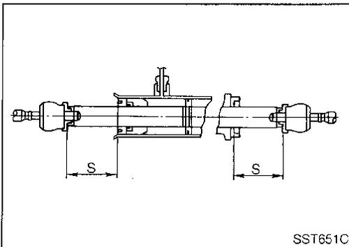
2. If it is not within specification, check rack stroke.
