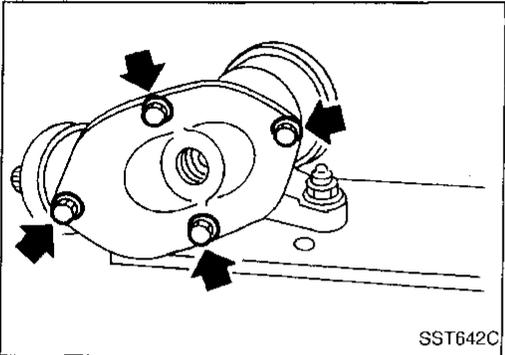
23. Install front cover using a new gasket.
