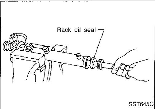
4. Install rack oil seal and rack bushing with rack assembly.
