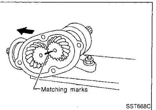
5. Wipe grease from the input and output gears.
