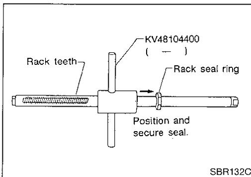
2. Using Tool, compress rack seal ring securely on rack.
