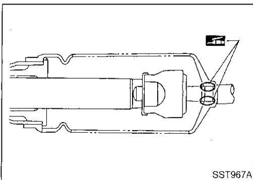
19. Before installing boot, coat the contact surfaces between boot and tie-rod with grease.
