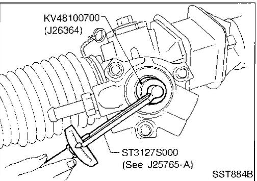
11. Measure pinion rotating torque.
