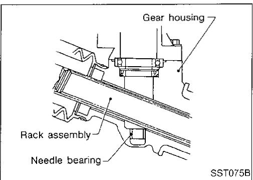
11. Apply a coat of multi-purpose grease to needle bearing roller and oil seal lip.
