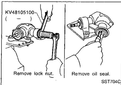
1. While holding inner nut using Tool, remove lock nut.
