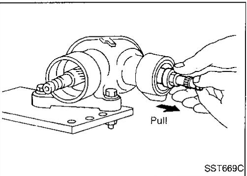
2. Insert input shaft until it comes in contact with end face of gear box.
