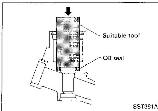
8. Coat seal lip of new pinion oil seal with multi-purpose grease. Install it into pinion housing of gear with a suitable tool.
