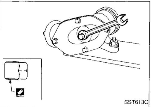
24. Apply liquid packing to threads of plug, and tighten it.
