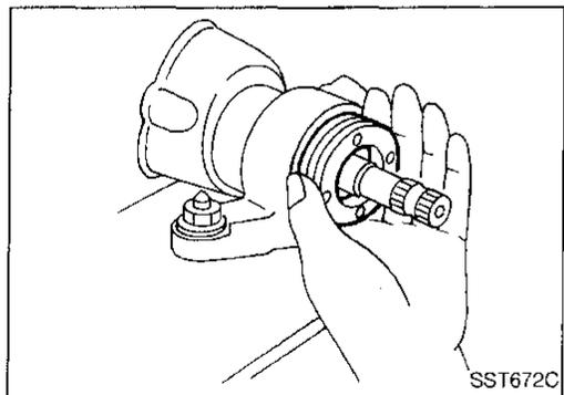
15. Install and hand tighten input shaft rear cover.
