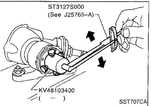
25. Measure rotating torque at input shaft.
