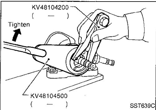
18. While holding rear cover with Tool (pin-type nut wrench), tighten lock nut with Tool.
