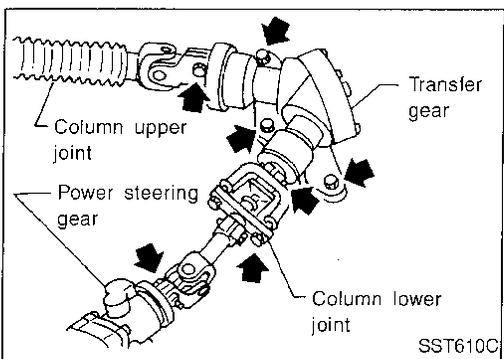
3. Remove steering column upper and lower joint from transfer gear.
