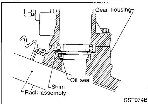
9. Install pinion bearing adjusting shim(s).
