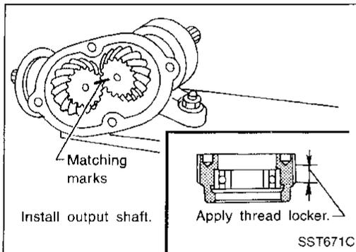
13. Align matching marks on gears made during disassembly step.
