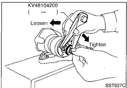
16. Tighten input shaft rear cover until input shaft meshes with output shaft.
