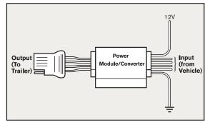
**CAUTION:** Do NOT connect the trailer wiring directly to the vehicle wiring. Splice the Input side of the Power Module/Converter into the vehicle wiring ONLY. See the below illustrations for the splicing locations.
