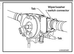
7. While pressing tabs, pull lighting and turn signal switch toward driver door and disconnect from base.
