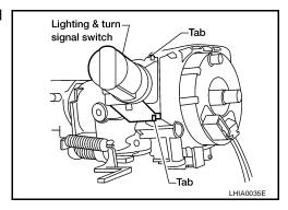
8. Remove the screws, release the clip, and remove the spiral cable.
