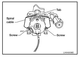
9. Remove the spiral cable connectors.
