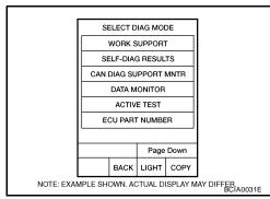
7. If no malfunction is detected on "SELF-DIAG [CURRENT]", repair of SRS is completed. Go to step 8.
