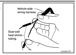
Fold each wire back and insert into the end of the heat shrink tubing so that the end of the wire is approximately centered in the heat shrink tubing.
