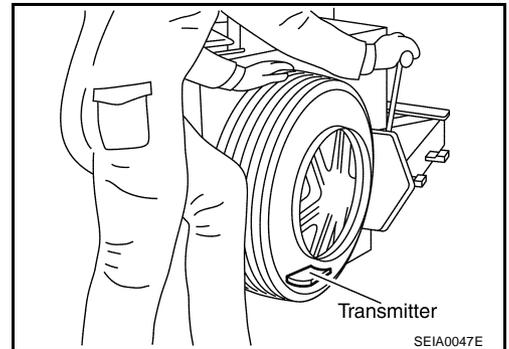
3. Turn tire so that valve hole is at bottom and bounce so that transmitter is near valve hole. Carefully lift tire onto turntable and position valve hole (and transmitter) 270 degree from mounting/dismounting head.
