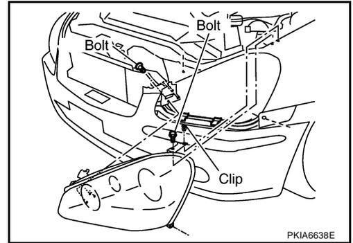
6. Pull the side of the front bumper toward the front of the vehicle and disengage it from clips on the body.
