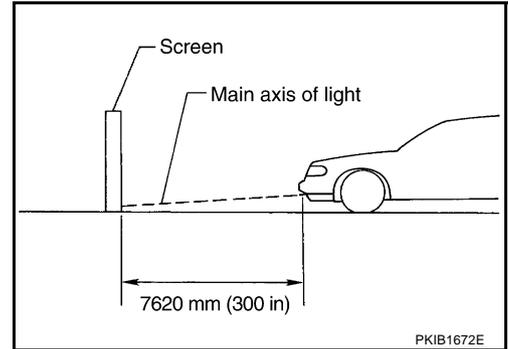
3. Adjust front fog lamps using adjusting screw so that the top edge of the high intensity zone is 100 mm (3.94 in) below the height of the fog lamp centers as shown.
