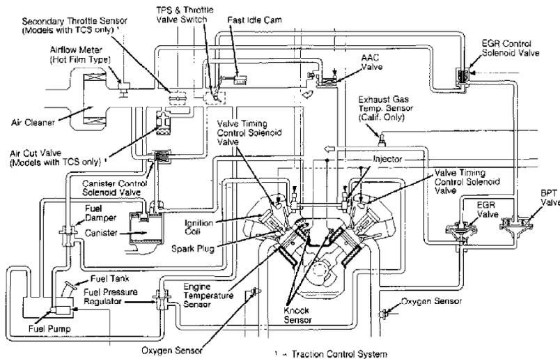
Fig. 3: Vacuum Diagram (Q45)
