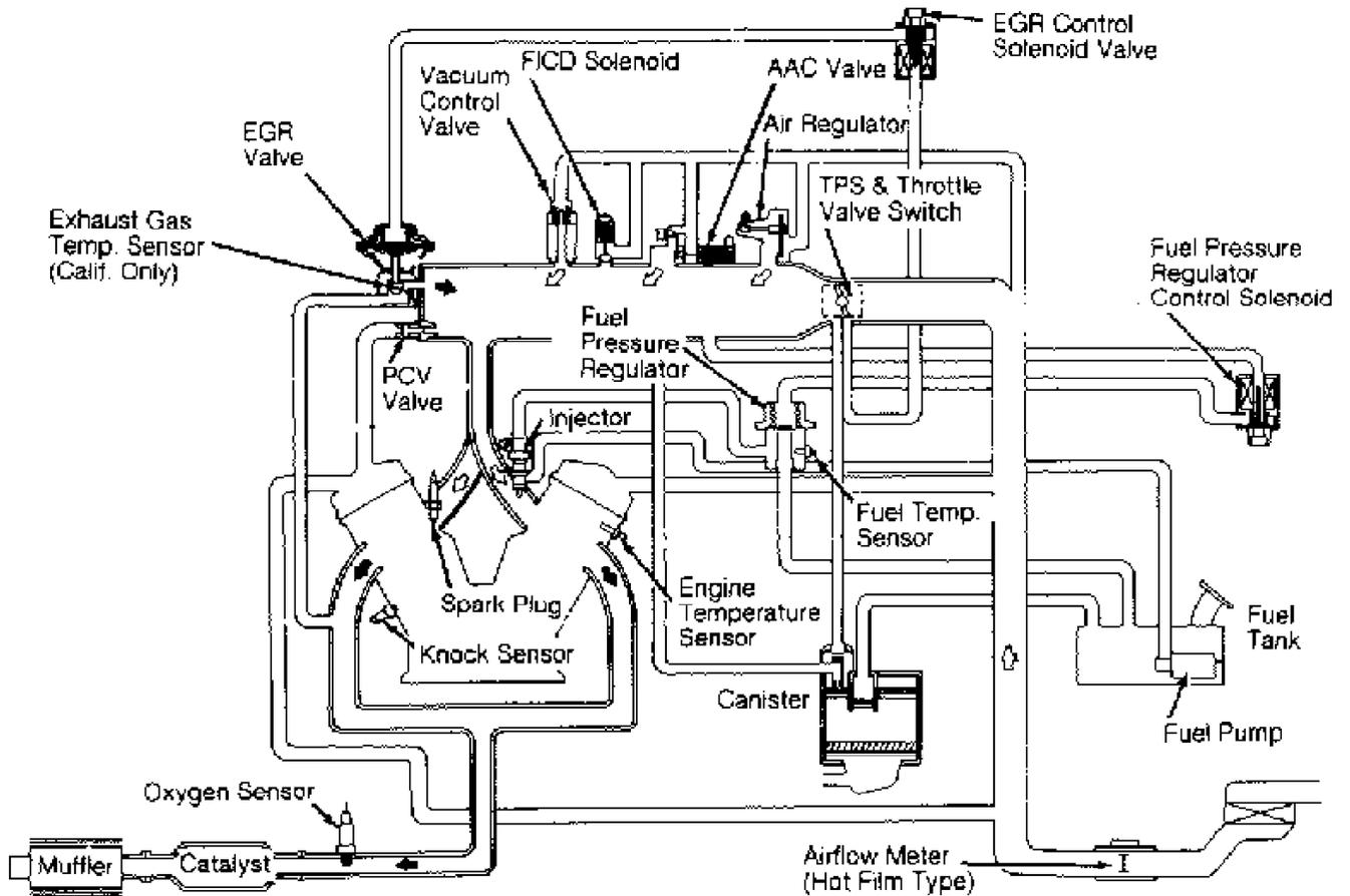
Fig. 2: Vacuum Diagram (M30)
