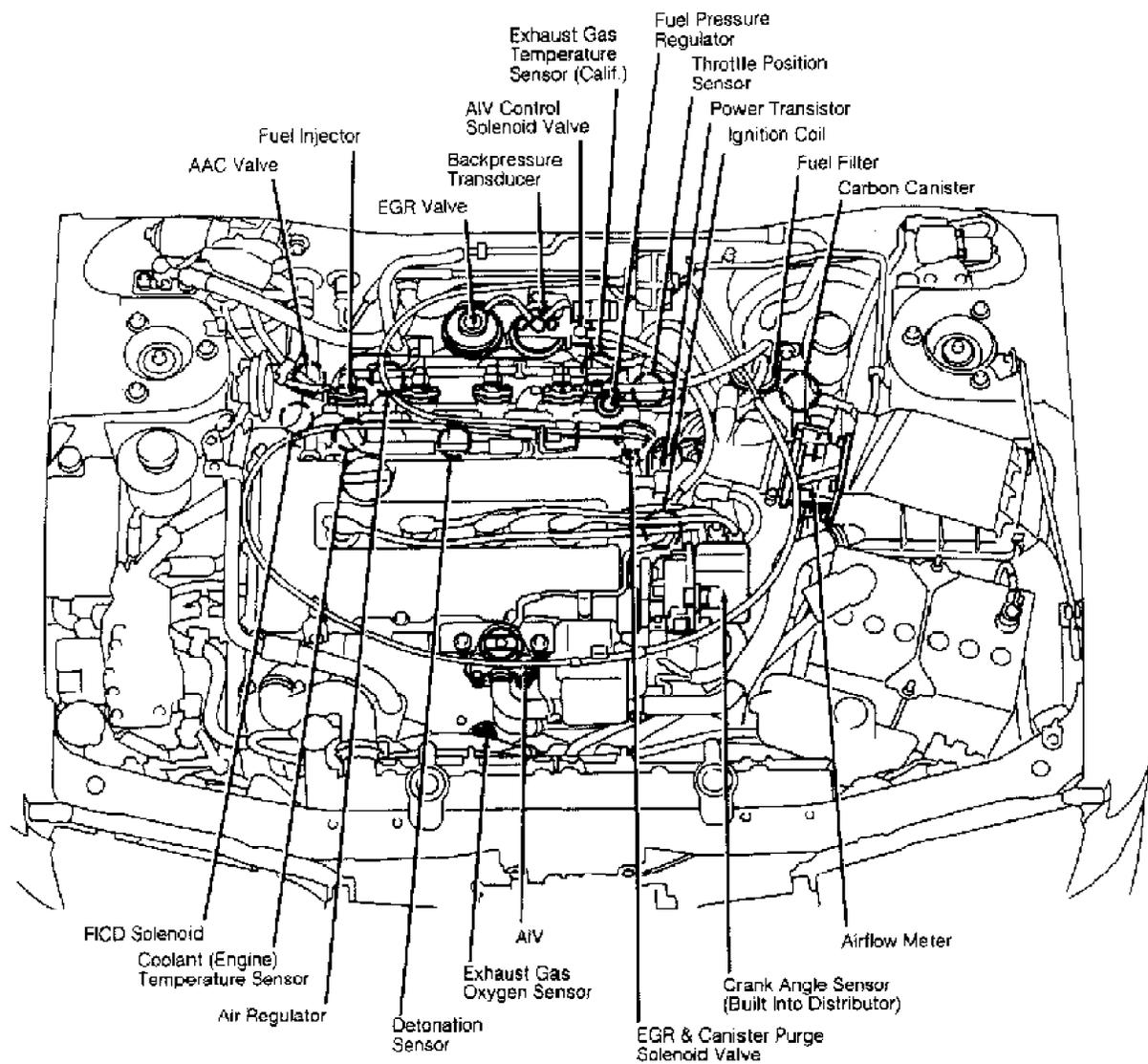
Fig. 17: Underhood Engine Performance Component Locations (G20)
