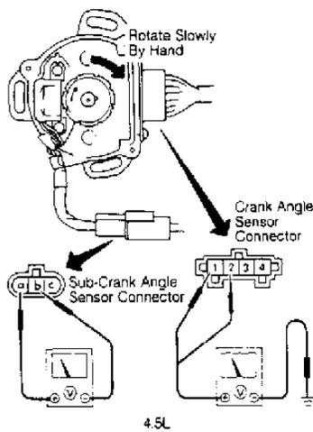
Fig. 6: Crankshaft Angle Sensor Terminal ID (Q45)
