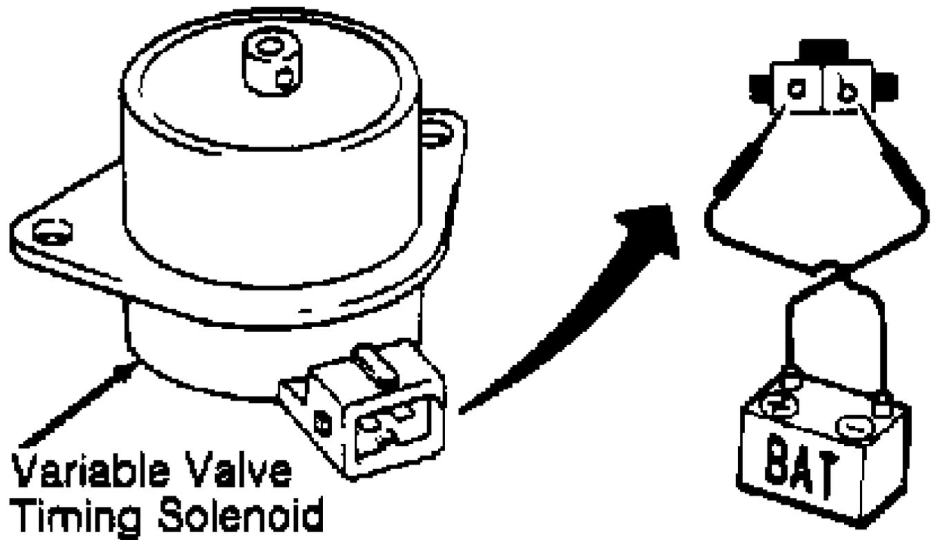
Fig. 16: Energizing Variable Valve Timing Solenoid
