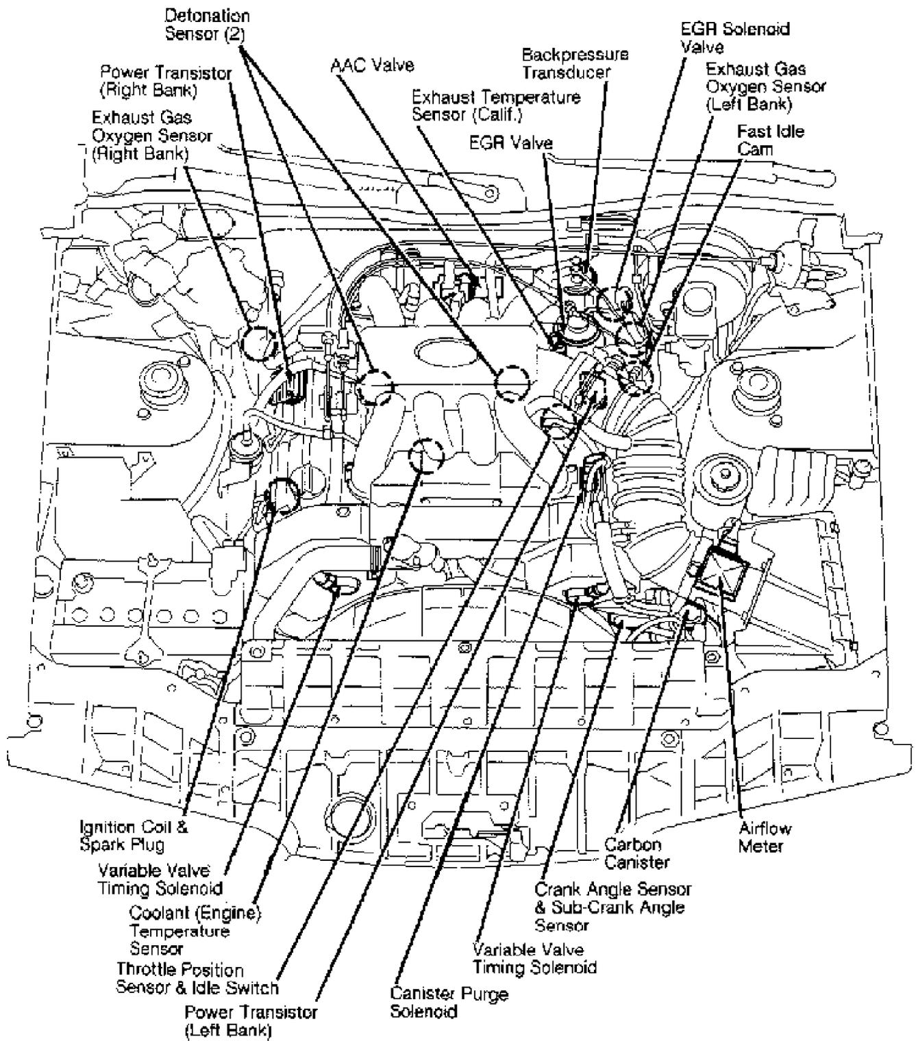
Fig. 19: Underhood Engine Performance Component Locations (Q45)
