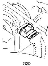
Fig. 2: Airflow Meter Connector ID (G20)
