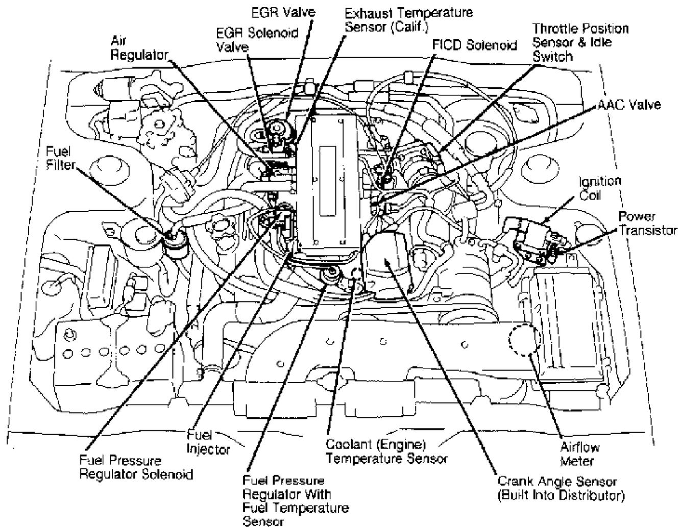
Fig. 18: Underhood Engine Performance Component Locations (M30)
