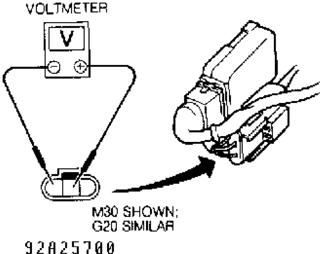
Fig. 3: Measuring Throttle Position Sensor Voltage (G20 & M30)
