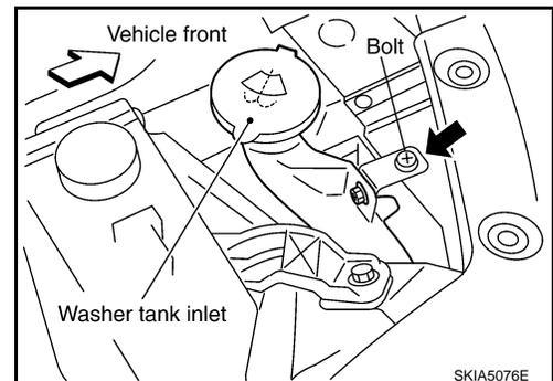
2. Remove front fillet molding (RH). Refer to [EI-14, "Component Parts Location"](#).
