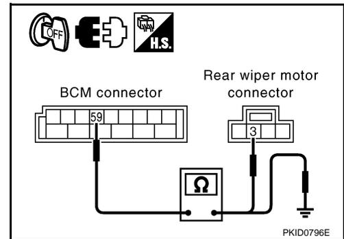
5. Check continuity between rear wiper motor harness connector and ground.
