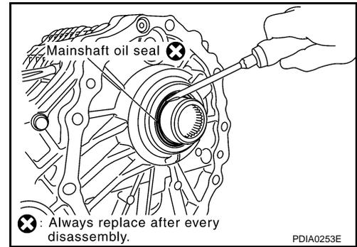
3. Remove front oil seal from front case, using a flat-bladed screwdriver.
