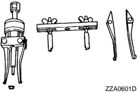
ZZA0601D                                                                                   | <ul style="list-style-type: none"> <li>Removing rear oil seal</li> </ul>                                          |
