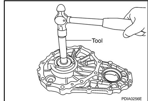
13. Remove drive chain and front drive shaft while tapping front drive shaft with plastic hammer.
