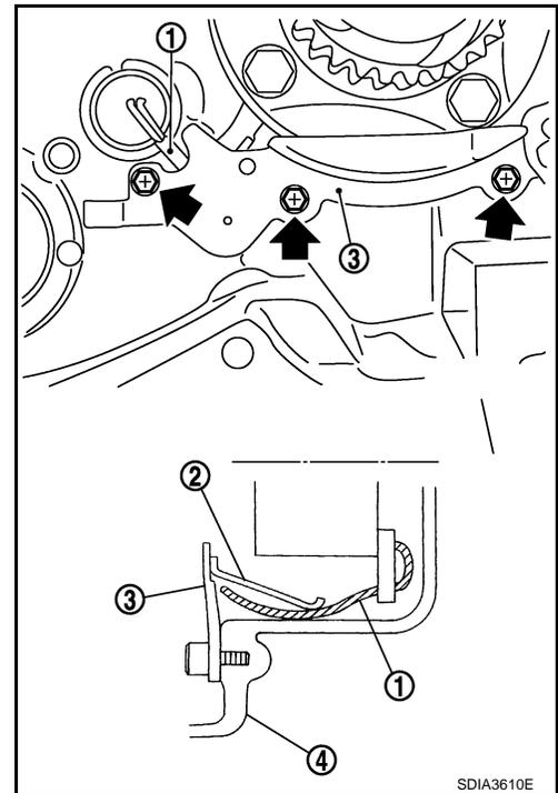
10. Install oil gutter to rear case.
