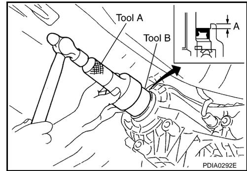
2. Align the matching mark of mainshaft with the mark of companion flange, then install the companion flange.
