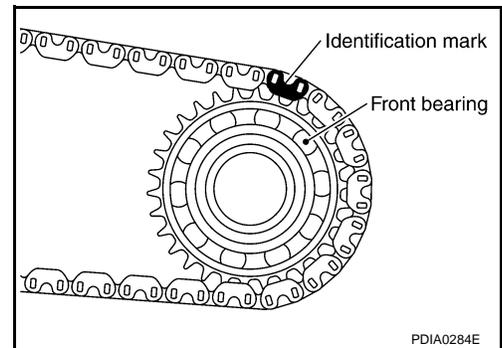
4. Install drive chain to mainshaft, and then install tap front drive shaft with plastic hammer. Press-fit rear bearing of front drive shaft to rear case.
