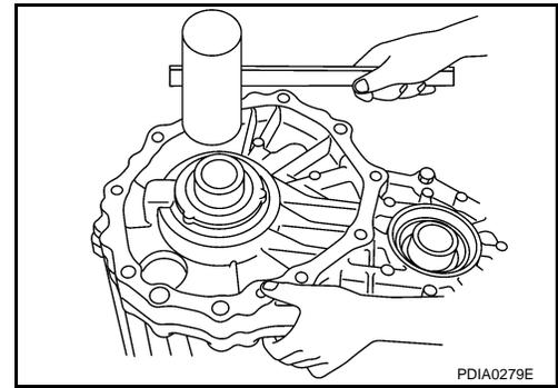
17. Tighten front case and rear case fixing bolts to the specified torque. Refer to "COMPONENTS".
