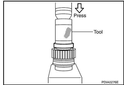
2. Install front drive shaft rear bearing, using a drift.
