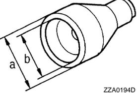
ZZA0194D                               | <ul style="list-style-type: none"> <li>Installing front oil seal</li> </ul>                                       |
