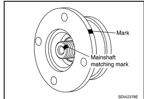
3. Using flange wrench, install the self-lock nut of companion flange and tighten to the specified torque. Refer to [TF-40, "Disassembly and Assembly"](#).
