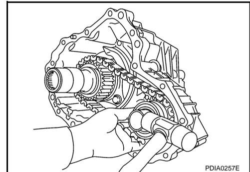
14. Remove oil gutter from rear case.
