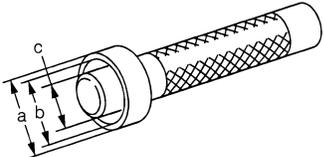
ZZA1046D | <ul style="list-style-type: none"> <li>Removing mainshaft bearing</li> </ul>                                      |
