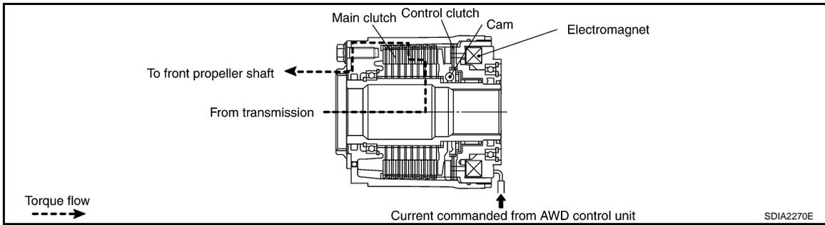
1. AWD control unit supplies command current to electric controlled coupling (AWD solenoid).
