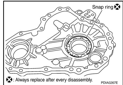
12. Remove mainshaft bearing from front case, using a drift.
