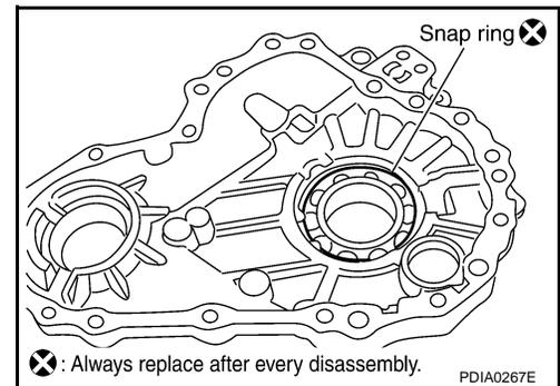
15. Apply liquid gasket to mating surface of rear case.
