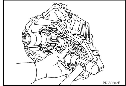
13. Install mainshaft bearing to front case, using a drift.
