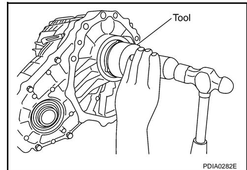
23. Install front oil seal until it is flush with end face of front case, using drift.
