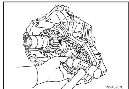
3. Remove front drive shaft front bearing, using drift and puller.
