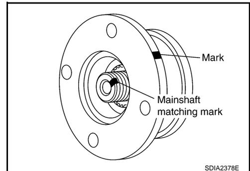
6. Remove companion flange, using a puller.
