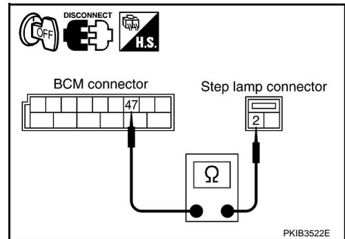
3. Check continuity between BCM harness connector and rear step lamp harness connector.
