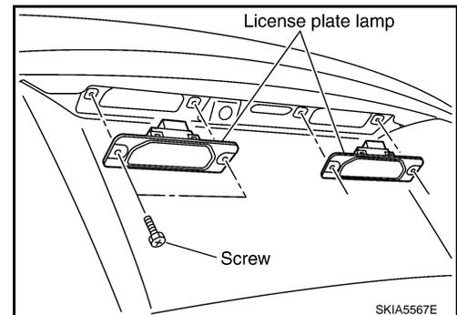
3. Insert a flat head or suitable tool and remove housing.
