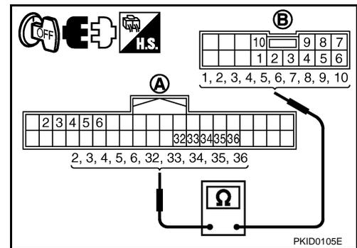
4. Check for continuity between each of BCM harness connector in suspect malfunctioning system and ground.
