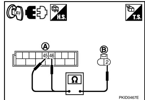
5. Check continuity between BCM harness connector (A) and rear combination lamp (RH and LH) harness connectors (B).
