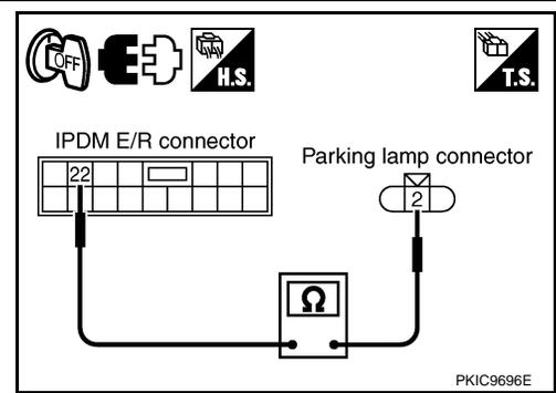
5. Check continuity between IPDM E/R harness connector and license plate lamp harness connector.
