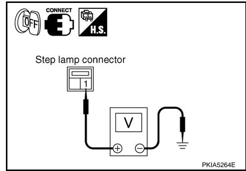
3. Check voltage between rear step lamp (LH and RH) harness connector and ground.
