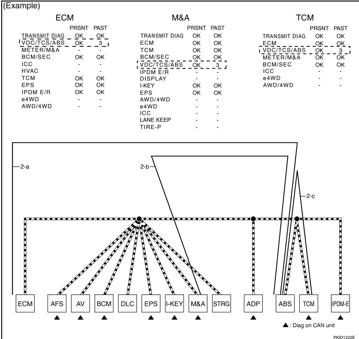
3. CAN DIAG SUPPORT MNTR (without PAST): Check the CAN DIAG SUPPORT MNTR (without PAST) of units indicating "U1000" or "U1001" on SELF-DIAG RESULTS. Draw a line on the diagnosis sheet to indicate the possible error circuit.
