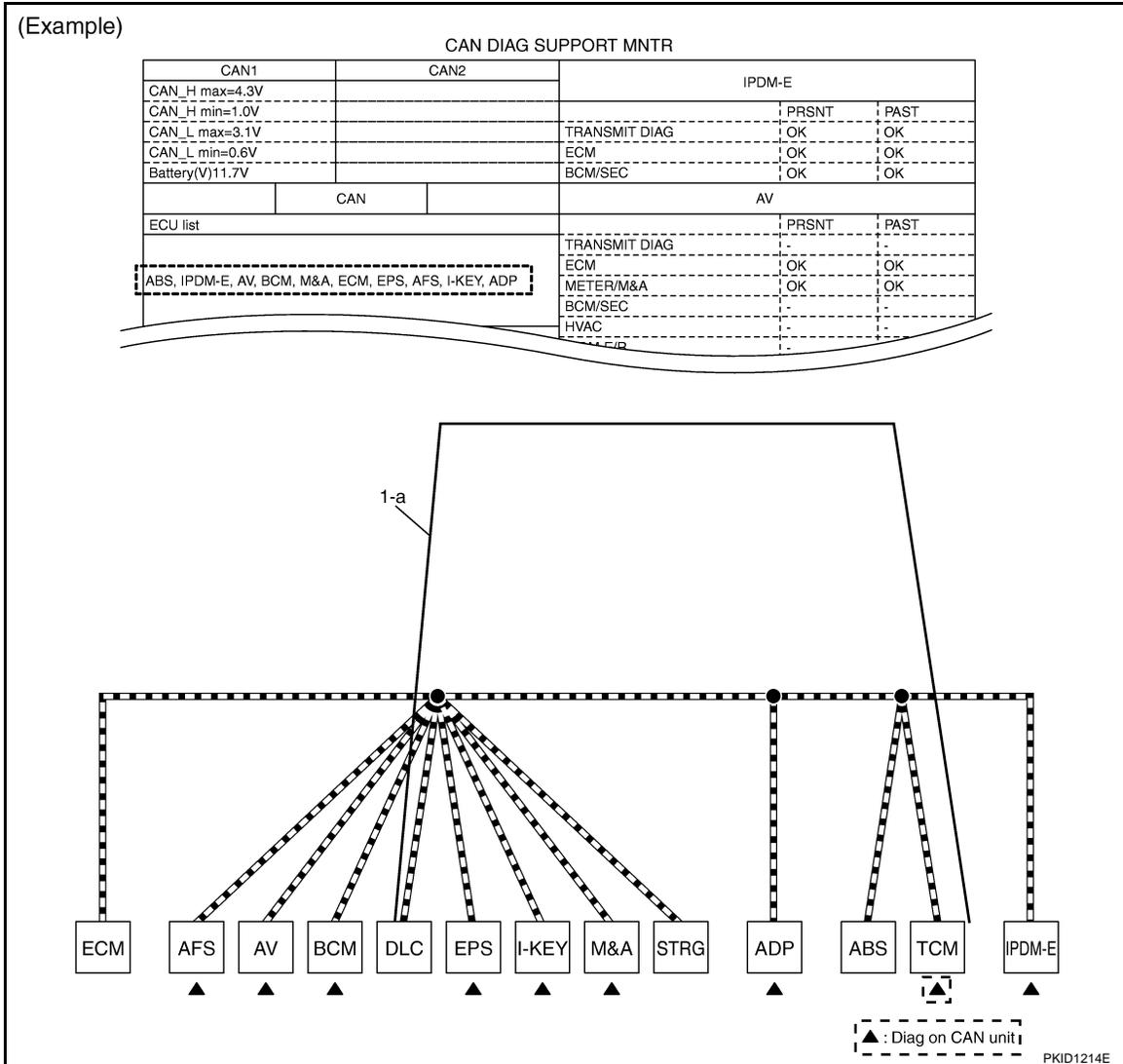
2. CAN DIAG SUPPORT MNTR: Check each item on “CAN DIAG SUPPORT MNTR”. Draw a line on the diagnosis sheet to indicate the error circuit.
