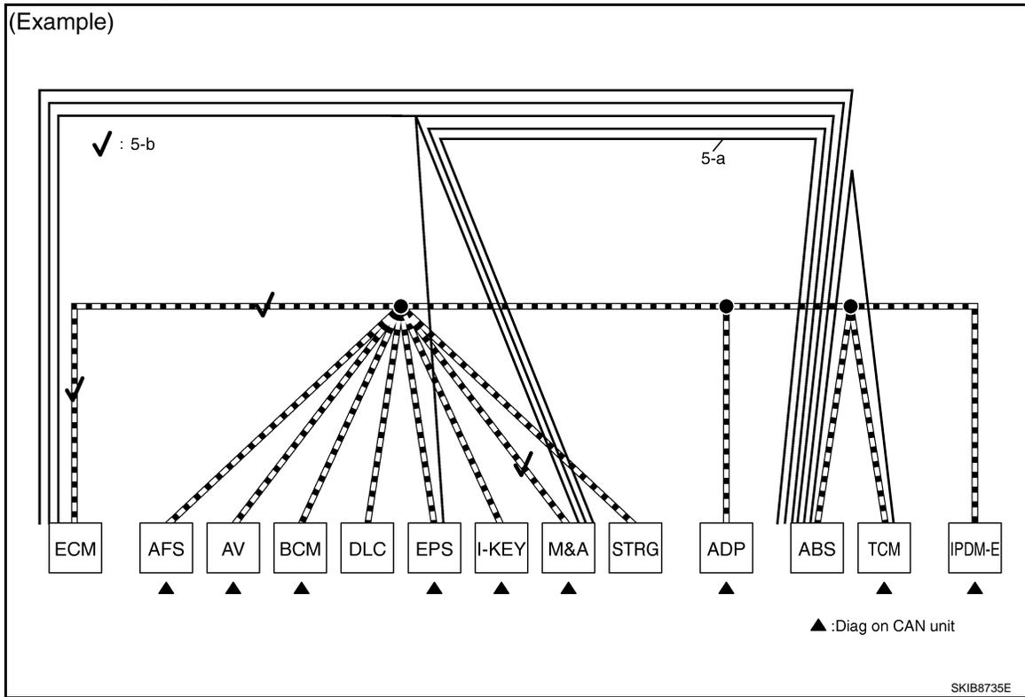
6. The circuit which has the most amount of lines are the possible cause. Error is detected from ABS actuator and electric unit (control unit) branch line (shaded in the figure below).
