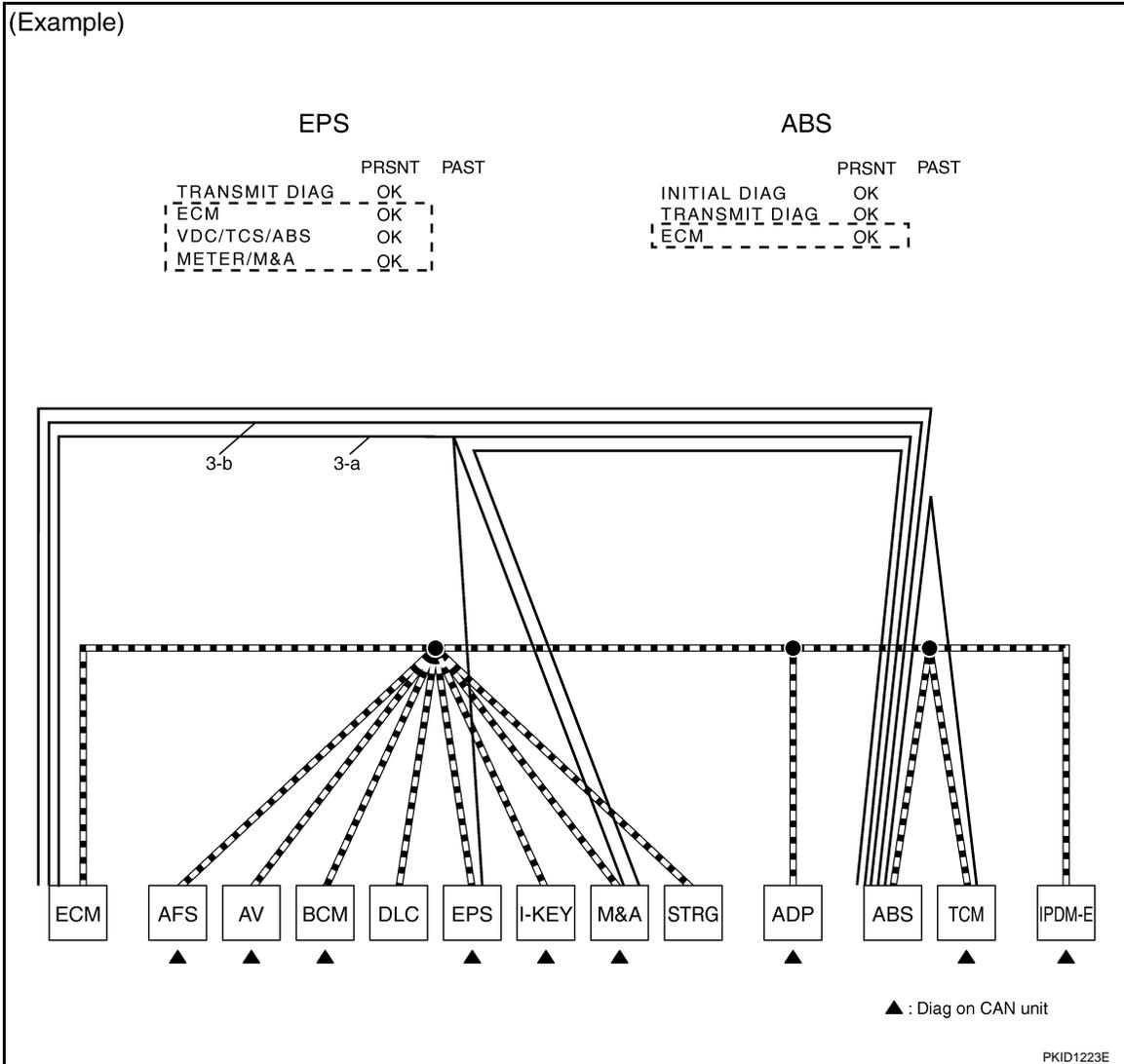
4. Search for the possible cause using CAN communication signal chart using information from the interview with the customer.
