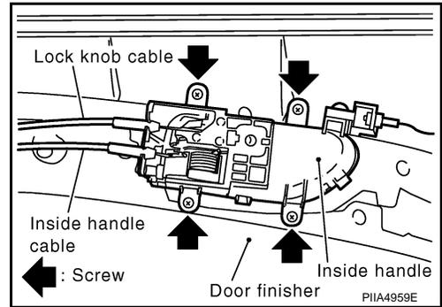
6. Remove the following parts after removing door finisher.
