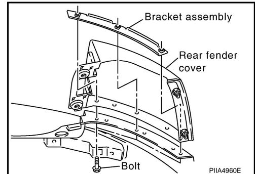
2. Remove bracket clips and remove bracket.
