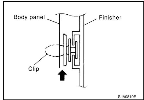
4. Pull up door finisher, and remove electrical parts connectors.
