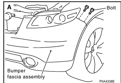
6. Insert driver rolled with cloth between bumper fascia and "S" type clips, and remove bumper fascia.
