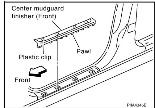
2. Remove center mudguard finisher clip and remove center mudguard finisher (rear).
