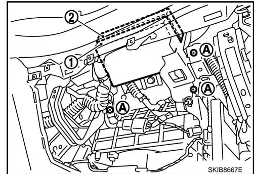
3. Remove TEL adapter unit screws, display control unit screws, and remove brackets.
