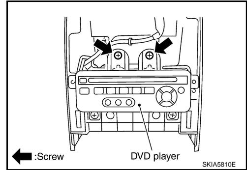
4. Remove screws (4) with power tool and remove brackets.
