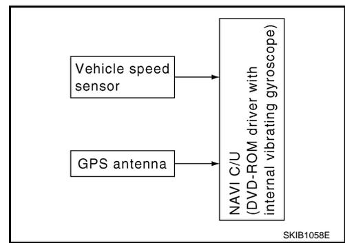
The current vehicle position will be calculated by detecting the distance the vehicle moved from the previous calculation point and its direction.
