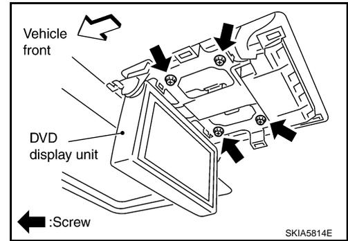
4. Pull DVD display unit to downside, and remove rear display unit from mounting plate.
