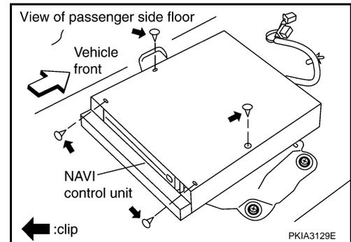
3. Remove screws (2) and nut (1) with power tool, and remove NAVI control unit.
