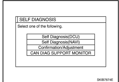
6. Each diagnosis is shown by selecting each screen switch on Confirmation/Adjustment screen.
