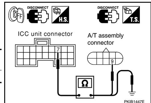
4. Check continuity between ICC unit harness connector and ground.
