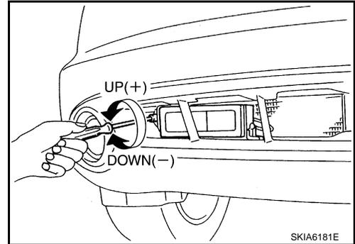
5. When “U/D CORRECT” value indicates  $\pm 4$ , confirm that the margin of value remains within  $\pm 4$  at least for 2 seconds with no equipment or hand touching the ICC sensor. When “COMPLETED THE VERTICAL AIMING OF LASER BEAM” appears on screen, touch “END”.
