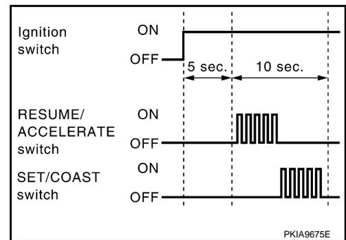
5. When self-diagnosis mode is started, DTC are shown on set vehicle speed indicator.
