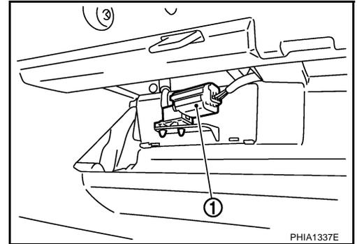
2. Remove glove box assembly and instrument passenger lower panel. Refer to [IP-11, "Removal and Installation"](#).
