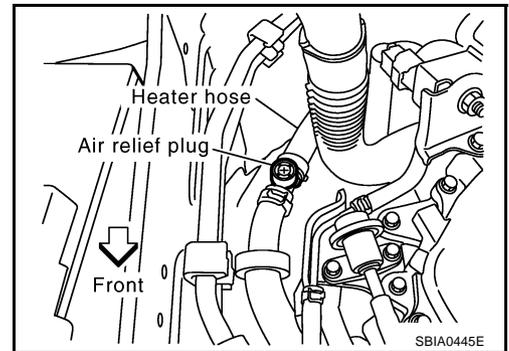
4. Fill radiator, and reservoir tank if removed, to specified level.
