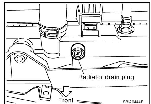
When draining all of engine coolant in the system, open water drain plugs on cylinder block. Refer to [EM-124. "DISASSEMBLY"](#).
