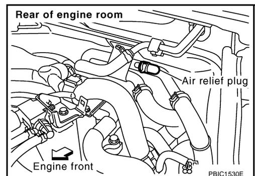
3. Fill thermostat housing with water until water spills from the air relief hole, then close air relief plug. Fill thermostat housing and reservoir tank with water and reinstall radiator cap.
