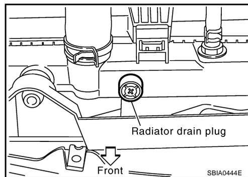
**When draining all of engine coolant in the system, open water drain plugs on cylinder block. Refer to [EM-249, "DISASSEMBLY"](#) .**
