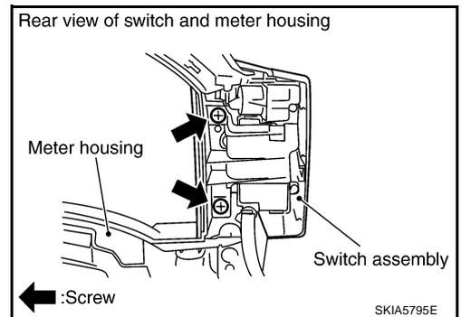
4. Remove screws (5), and remove odo/trip meter and illumination control switch.
