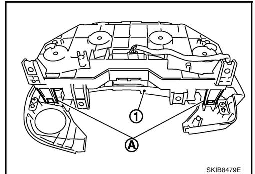
5. Remove screws (A) and remove reinforcing metal (1).
