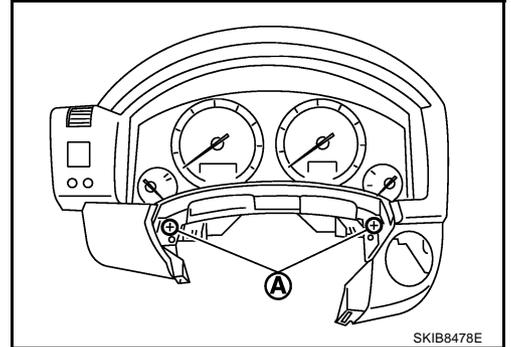
4. Remove tabs (A) and remove switch and meter housing (1).
