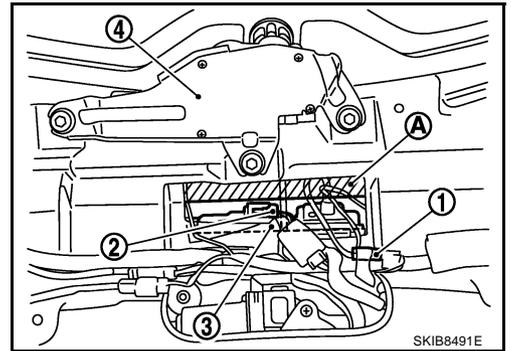
8. Remove screws (A), and remove rear view camera (1) from back door opener switch (2).
