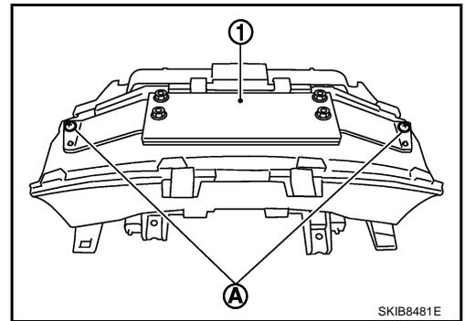
7. Disengage tabs (A) to separate front cover (1).
