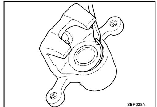
4. Place a wooden block as shown in the figure, and blow air from union bolt mounting hole to remove pistons and piston boots.
