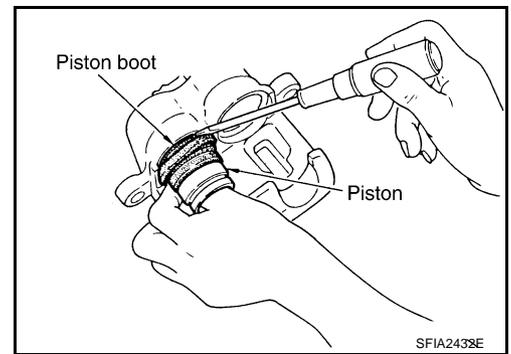
3. Apply brake fluid to piston, and press piston into cylinder body by hand to assemble piston side lip on piston boot properly into groove on piston.
