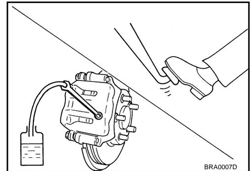
3. Make sure there is no foreign material in reservoir tank, and refill with new brake fluid.
