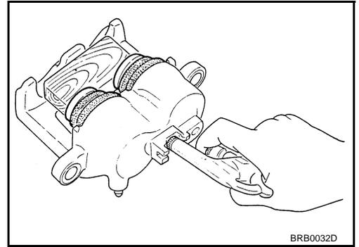
5. Using a flat-bladed screwdriver, remove piston seal from cylinder body.
