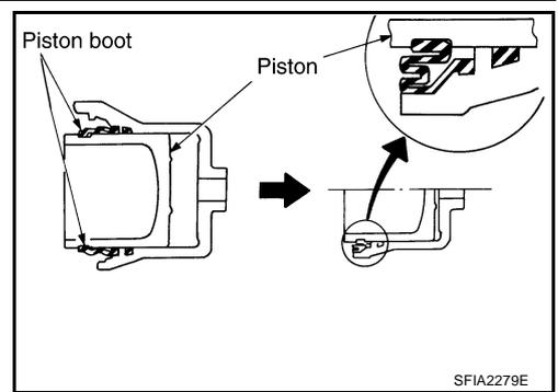
4. Fix piston boot with retaining ring.
