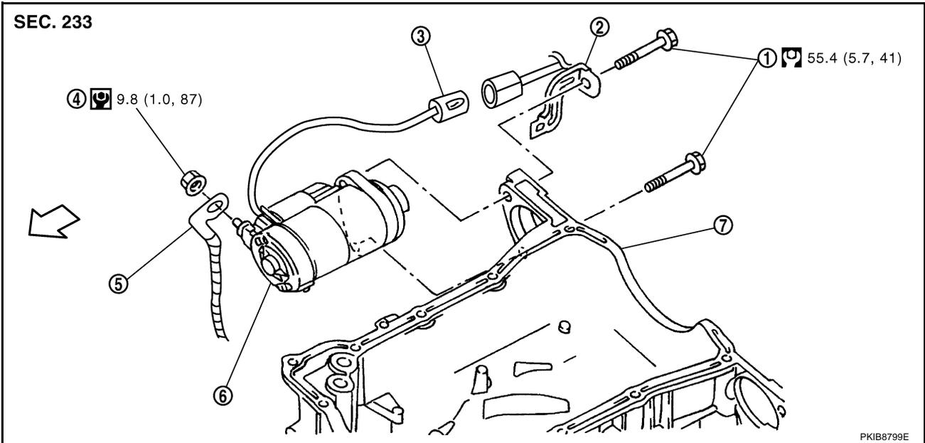
1. Starter motor mounting bolt
