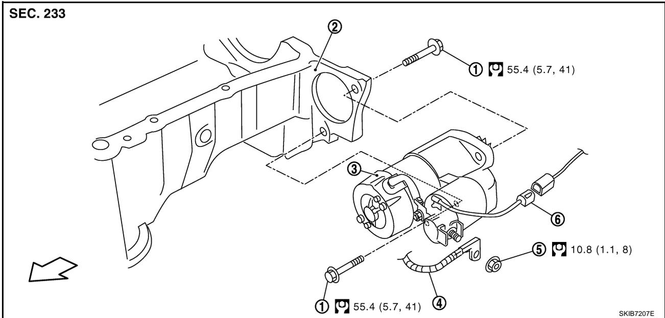
1. Starter motor mounting bolt
