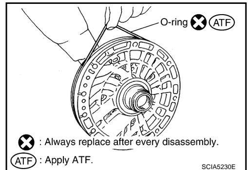
2. Install O-ring to oil pump housing.
