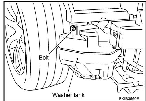
7. Remove washer tube, and remove washer tank from the vehicle.
