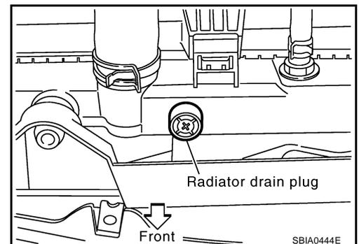
When draining all of engine coolant in the system, open water drain plugs on cylinder block. Refer to [EM-123. "DISASSEMBLY"](#).
