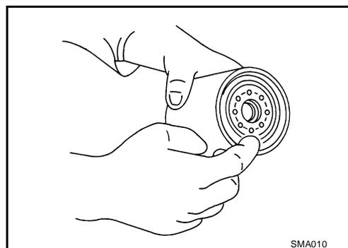
3. Screw oil filter manually until it touches the installation surface, then tighten it by 2/3 turn. Or tighten to specification.
