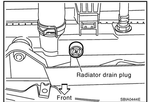
**When draining all of engine coolant in the system, open water drain plugs on cylinder block. Refer to [EM-246, "DISASSEMBLY"](#) .**
