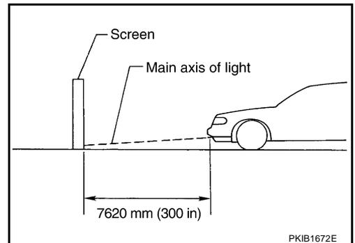
3. Adjust front fog lamps using adjusting screw so that the top edge of the high intensity zone is 100 mm (3.94 in) below the height of front fog lamp centers as shown at left.
