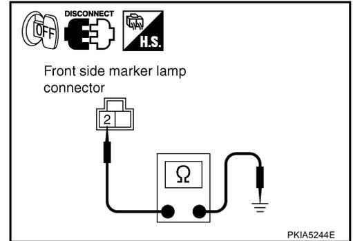
3. Check continuity between clearance lamp harness connector and ground.
