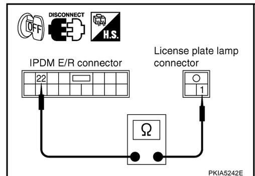
6. Check continuity between IPDM E/R harness connector and rear combination lamp harness connector.
