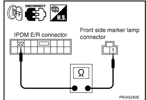
4. Check continuity between IPDM E/R harness connector and clearance lamp harness connector.
