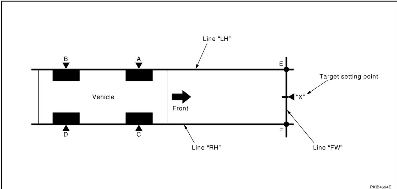
1. Mark a point at the center of lateral surface of each wheels ("A", "B", "C" and "D").
