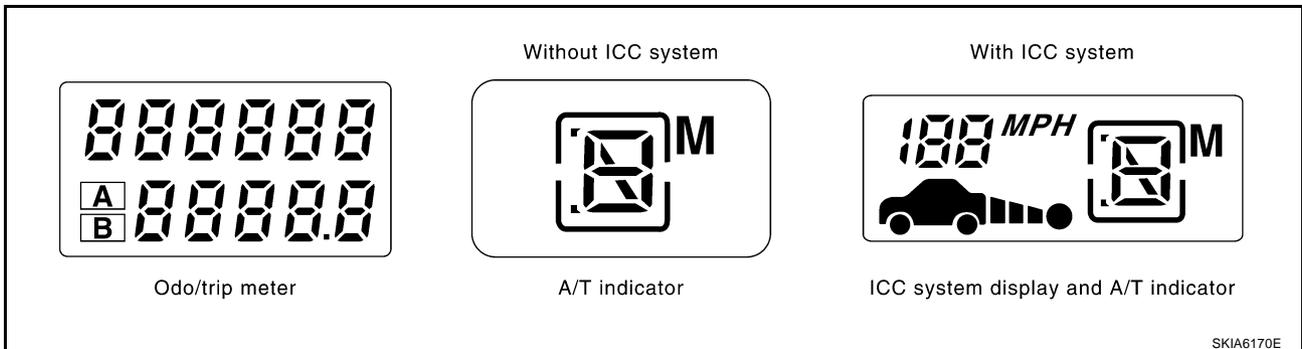
6. Push the trip reset switch. Each meter/gauge should indicate as shown in the figure while pushing trip reset switch. (At this time, the low-fuel warning lamp goes off.)
