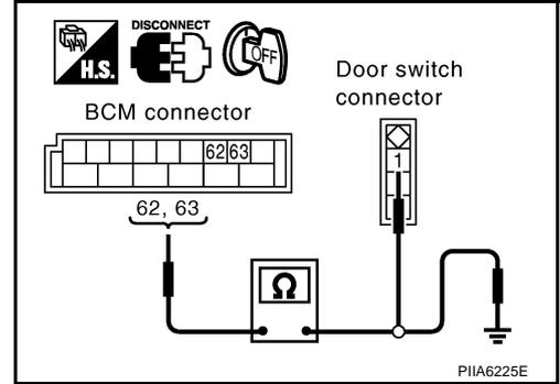
4. Check continuity between BCM connector M3 terminals 12, 13 and door switch connector B36, B206 terminal 1, and ground.
