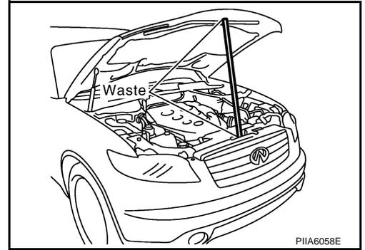
2. Remove the hood stays from the stud balls on the body side.
