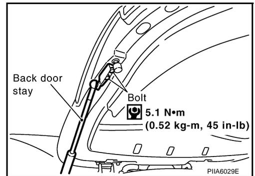
3. Remove back door stay assembly on vehicle.
