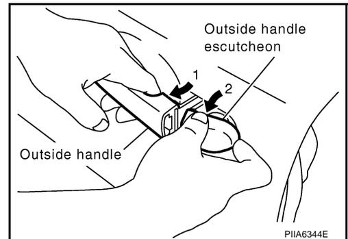
6. While pulling outside handle, slide toward rear of vehicle to remove outside handle.
