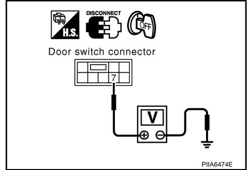
4. Check continuity between back door switch connector D109 terminal 7 and ground. (Check harness for short.)
