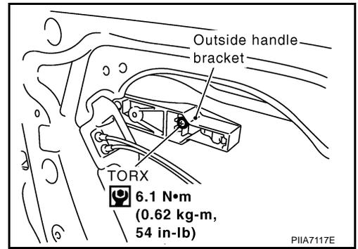
9. While pulling outside handle, slide toward front of vehicle to remove outside handle bracket.
