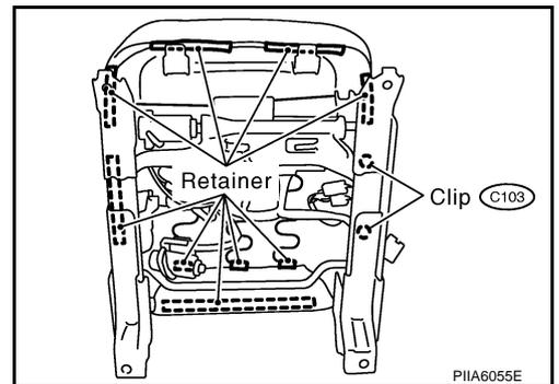
8. After removing the seat cushion trim and pad, remove the hog rings to separate the trim and pad and the seat cushion heater unit.
