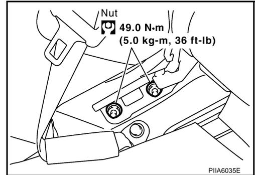
3. Remove the seatback mounting bolt and nut.
