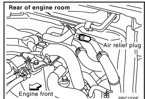
3. Fill thermostat housing with water until water spills from the air relief hole, then close air relief plug. Fill thermostat housing and reservoir tank with water and reinstall radiator cap.
