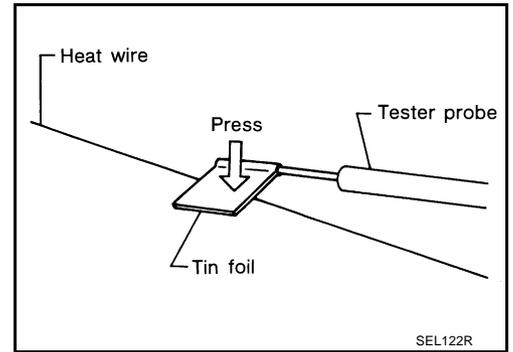
2. Attach probe circuit tester (in Volt range) to middle portion of each filament.
