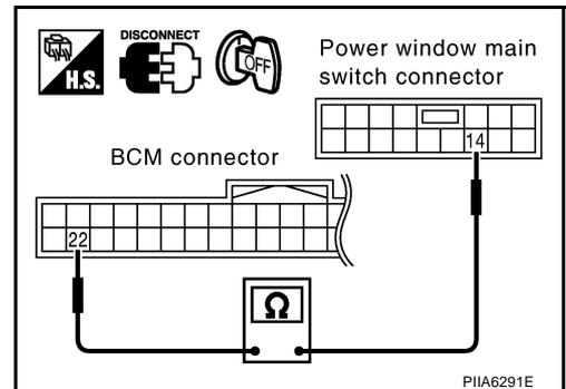
3. Check continuity between BCM connector M3 terminal 22 and front power window switch (passenger side) connector D36 terminal 16.
