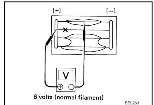
3. If a filament is burned out, circuit tester registers 0 or battery voltage.
