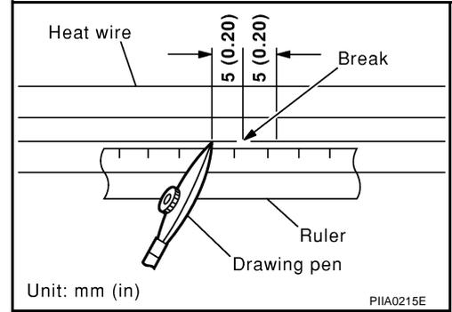
4. After repair has been completed, check repaired wire for continuity. This check should be conducted 10 minutes after silver composition is deposited. Do not touch repaired area while test is being conducted.
