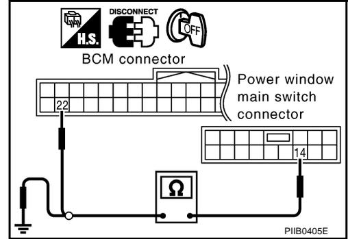
5. Check continuity between BCM connector M3 terminal 22 and front power window switch (door lock and unlock switch) connector D36 terminal 16.
