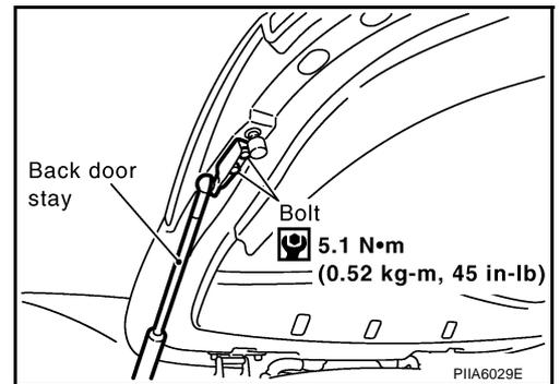
3. Remove back door stay assembly on vehicle.
