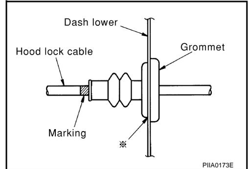
4. Install the cable securely to the lock.
