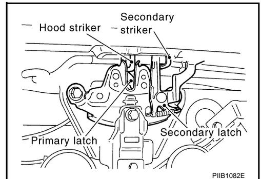
3. When pulling hood opener lever gently, make sure that front end of the hood rises by approximately 20 mm (0.79 in) and that hood striker and hood lock primary latch are disengaged. Also make sure that hood opener returns to the original position.
