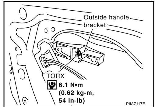
11. While pulling outside handle bracket, slide toward front of vehicle to remove outside handle bracket.
