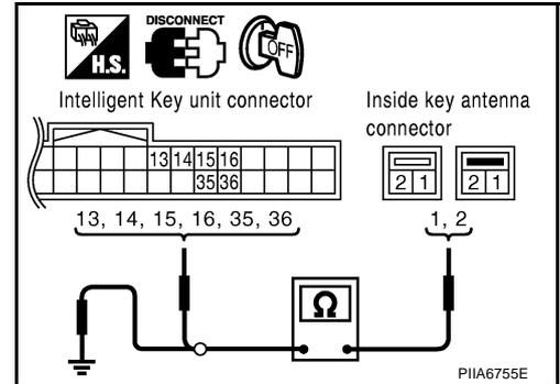
3. Check continuity between inside key antenna connector M70, M153 (dash board), B68 (luggage room) terminals 1 and 2 and ground.
