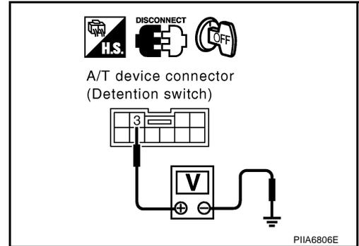
3. Check continuity between A/T device (detention switch) connector M67 terminals 3 (R/Y) and ground. (Check harness for short.)
