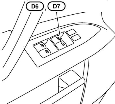
Front power window switch (passenger side) (door lock and unlock switch)
