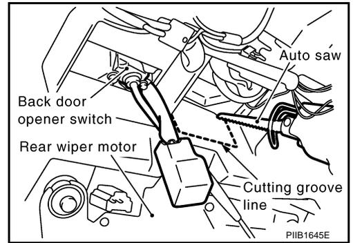
5. Disconnect back door opener switch harness connector (and rear view camera if equipped).
