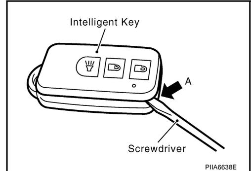
3. When replacing the circuit board or rubber
