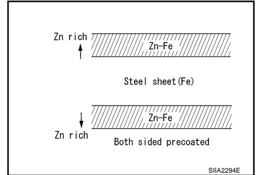
Nissan Genuine Service Parts are fabricated from galvannealed steel. Therefore, it is recommended that GENUINE NISSAN PARTS or equivalent be used for panel replacement to maintain the anti-corrosive performance built into the vehicle at the factory.
