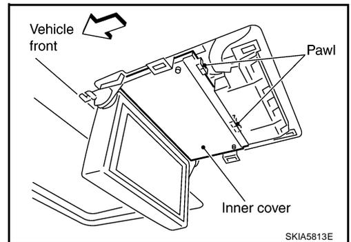
3. Remove screws (4) with power tool.
