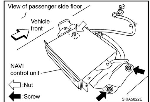
4. Remove screws (4) with power tool and remove bracket.
