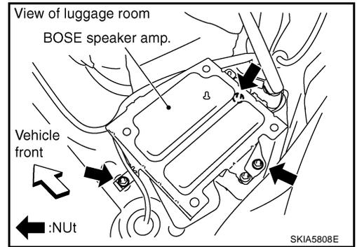
3. Remove nuts (2) with power tool, and remove assist bracket.
