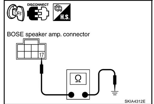
3. Check continuity between woofer harness connector B223 terminal 2 (B) and ground.
