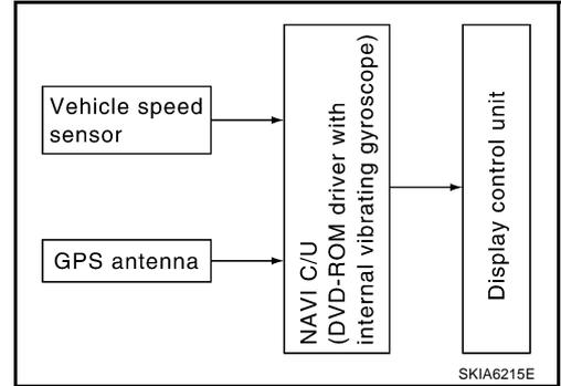
By comparing the vehicle position detection results found by the GPS and by map-matching, more accurate vehicle position data can be used.
