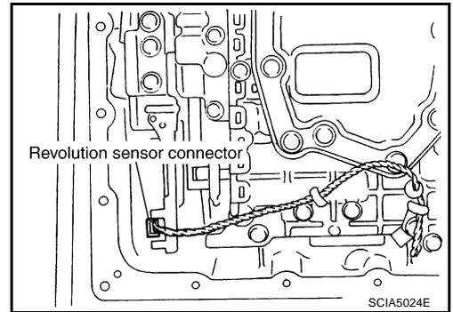
13. Securely fasten revolution sensor harness with terminal clips.
