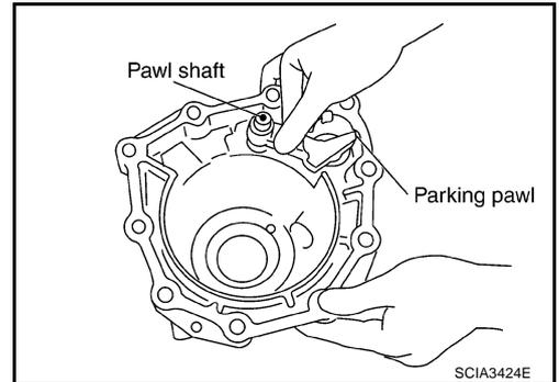
28. Install parking actuator support to rear extension (2WD models) or adapter case (AWD models).
