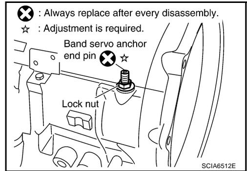
15. Remove brake band from transmission case.
