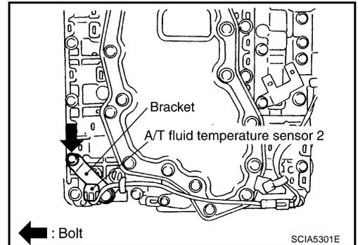
18. Remove bracket from A/T fluid temperature sensor 2.
