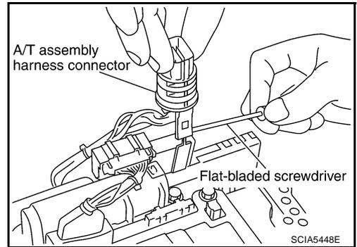
22. Disconnect TCM connector and park/neutral position switch connector.
