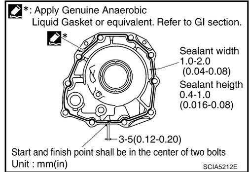
5. Install rear extension assembly to transmission case. (With needle bearing.)
