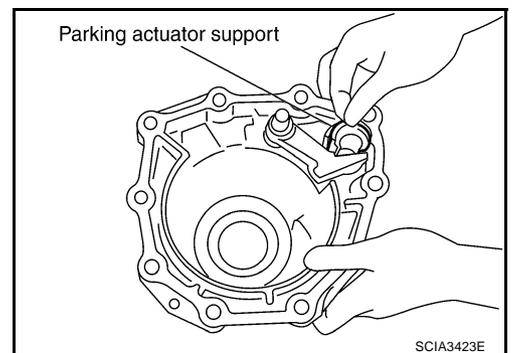
15. Remove parking pawl (with return spring) and pawl shaft from rear extension.
