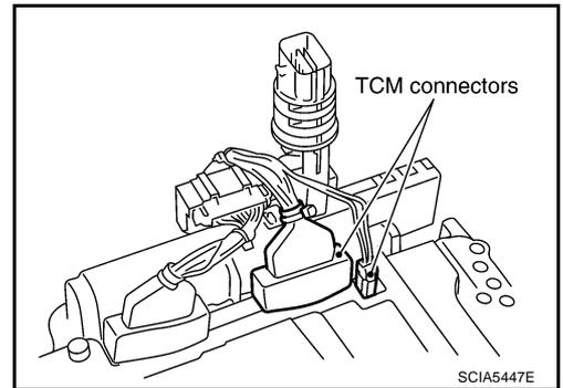
41. Remove A/T assembly harness connector from control valve with TCM using a flat-bladed screwdriver.
