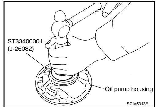
4. Install oil pump housing to oil pump cover.
