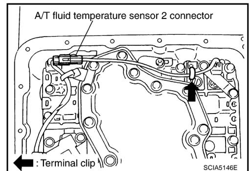
9. Remove A/T fluid temperature sensor 2 with bracket from control valve with TCM.
