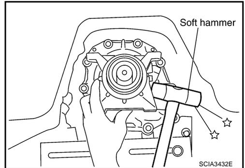
8. Remove rear extension assembly from transmission case. (With needle bearing.)
