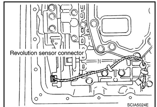
13. Securely fasten revolution sensor 2 harness with terminal clips.
