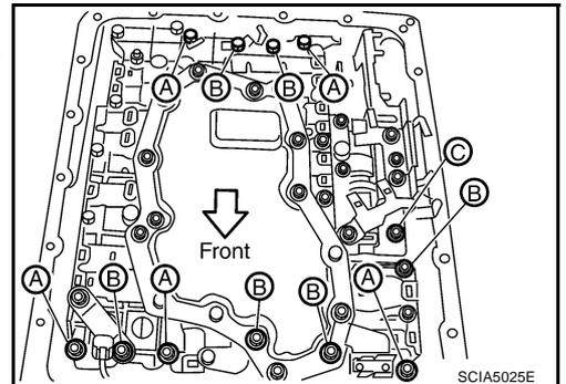
i. Tighten bolt 1, 2 and 3 temporarily to prevent dislocation. After that tighten them in order (1 → 2 → 3), and then tighten other bolts.
