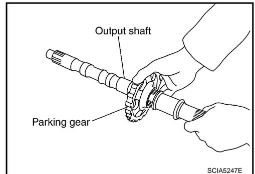
8. Install output shaft to transmission case.
