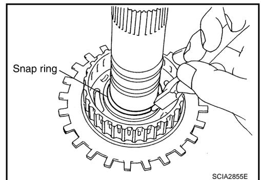
8. Check operation of 1st one-way clutch.
