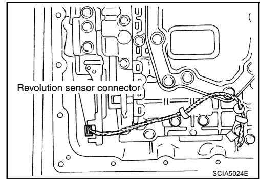
34. Straighten terminal clips to free revolution sensor harness.
