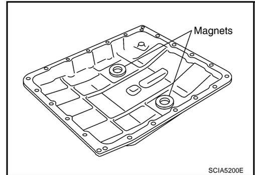
17. Install oil pan to transmission case.
