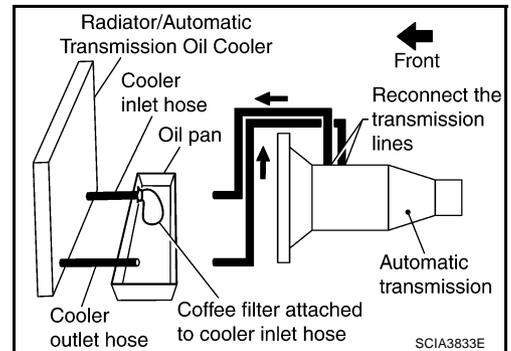
6. Insert the tip of an air gun into the end of the cooler outlet hose.
