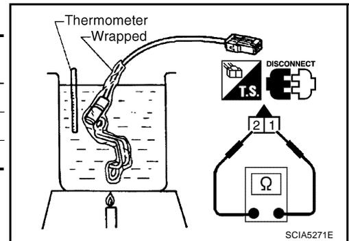
3. If NG, replace the A/T fluid temperature sensor 2. Refer to [AT-252, "A/T FLUID TEMPERATURE SENSOR 2 REMOVAL AND INSTALLATION"](#) .
