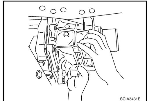
12. Tighten rear extension assembly mounting bolts to specified torque.
