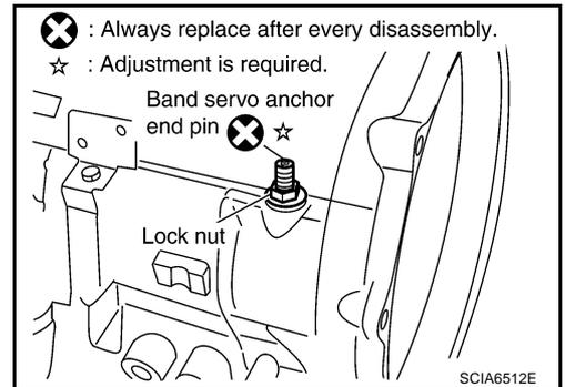
49. Install brake band in transmission case.
