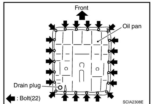
9. Check foreign materials in oil pan to help determine causes of malfunction. If the A/T fluid is very dark, smells burned, or contains foreign particles, the frictional material (clutches, band) may need replacement. A tacky film that will not wipe clean indicates varnish build up. Varnish can cause valves, servo, and clutches to stick and can inhibit pump pressure.
