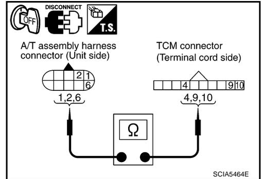
4. Check continuity between A/T assembly harness connector terminals and TCM connector terminals.
