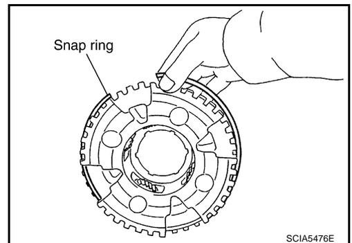
4. Disassemble input clutch assembly.
