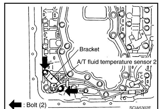
10. Remove bracket from A/T fluid temperature sensor 2.
