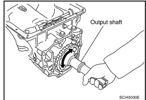
33. Install bearing race to output shaft.
