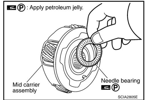
19. Remove needle bearing (rear side) from mid carrier assembly.
