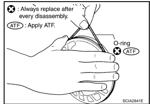
4. Remove O-ring from oil pump cover.
