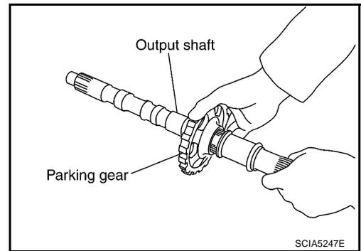
32. Install output shaft in transmission case.
