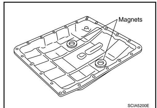
15. Install oil pan to transmission case.
