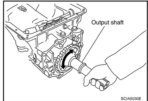
46. Remove parking gear from output shaft.
