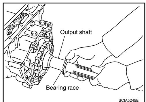
10. Remove output shaft from transmission case by rotating left/right.
