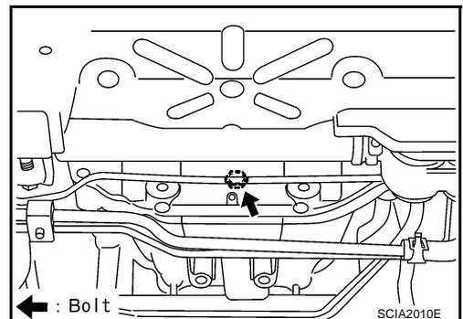
16. Remove dynamic damper (for VQ35DE models). Refer to [EM-110, "Removal and Installation"](#).
