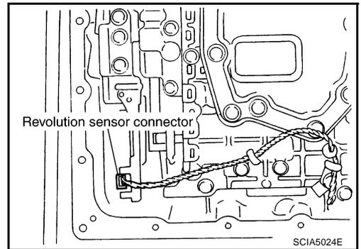
14. Straighten terminal clips to free revolution sensor harness.
