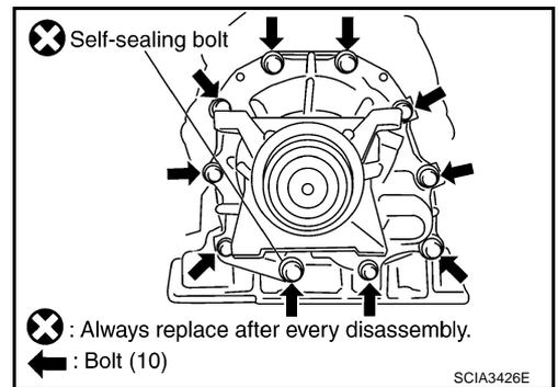
11. Tap rear extension assembly with soft hammer.
