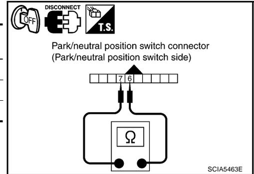
3. If NG, replace the control valve with TCM. Refer to [AT-244, "Control Valve with TCM and A/T Fluid Temperature Sensor 2"](#) .
