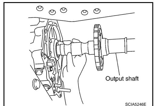
9. Install bearing race to output shaft.
