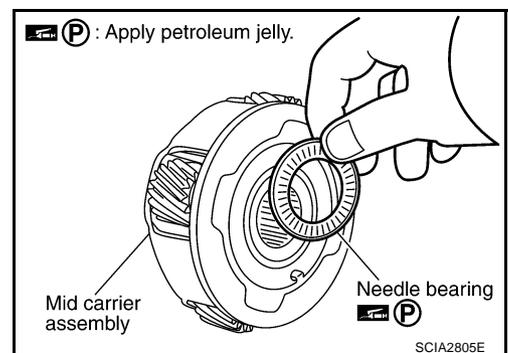
45. Install mid carrier assembly in rear carrier assembly.
