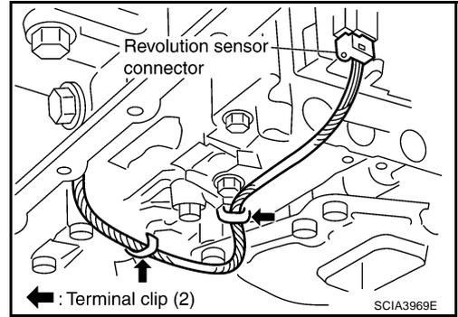
15. Remove revolution sensor from transmission case.
