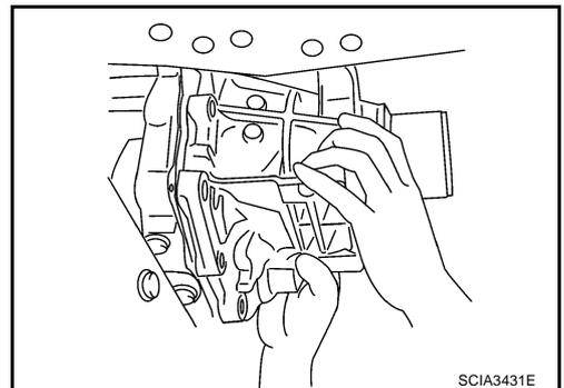
9. Remove bearing race from output shaft.
