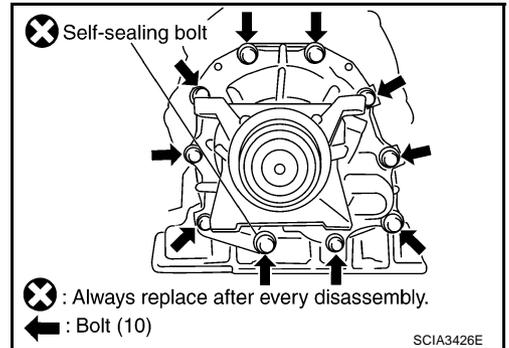
ii. Tap rear extension assembly with soft hammer.
