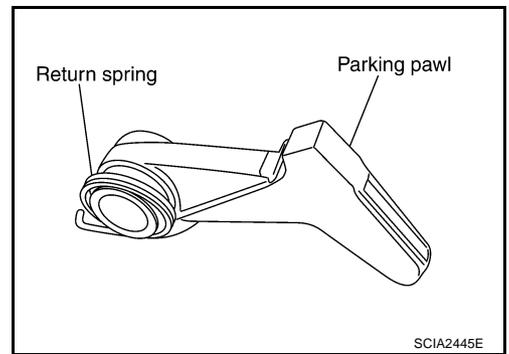
27. Install parking pawl (with return spring) and pawl shaft to rear extension (2WD models) or adapter case (AWD models).
