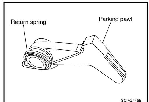
3. Install parking pawl (with return spring) and pawl shaft to rear extension.
