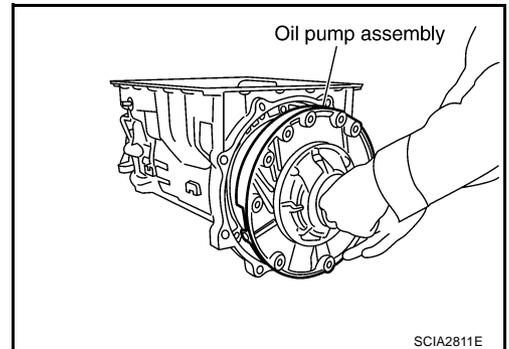
4. Apply recommended sealant (Genuine RTV Silicone Sealant or equivalent. Refer to [GI-48, "Recommended Chemical Products and Sealants"](#) .) to oil pump assembly as shown in illustration.
