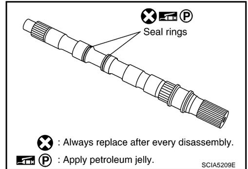
7. Install parking gear to output shaft
