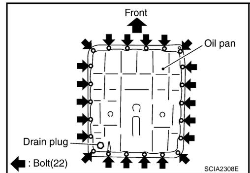
c. Tighten oil pan mounting bolts to the specified torque in numerical order shown in the figure after temporarily tightening them.
