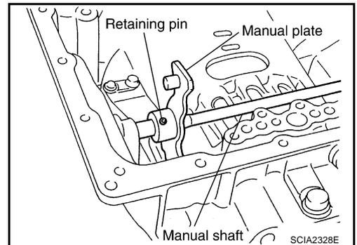
61. Remove manual shaft retaining pin with nippers.
