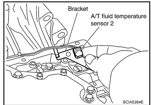
6. Install A/T fluid temperature sensor 2 (with bracket) in control valve with TCM.
