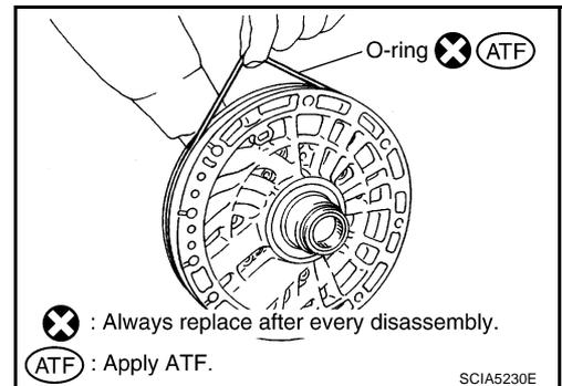
2. Install O-ring to oil pump housing.
