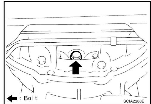
17. Remove engine rear member with power tool.
