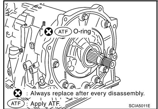
7. Install converter housing to transmission case.
