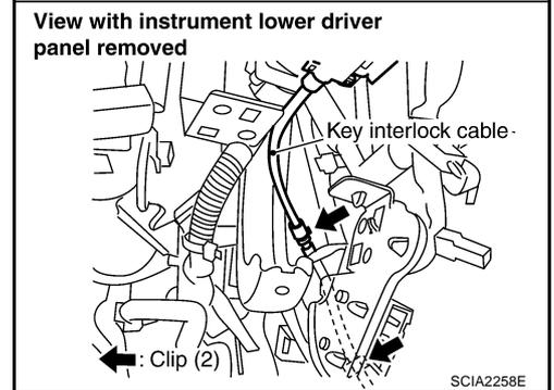
5. Insert interlock rod into adjuster holder.
