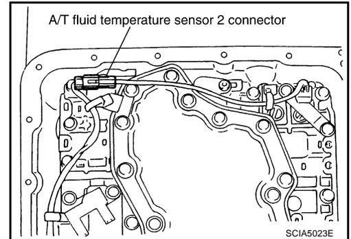
8. Straighten terminal clip to free A/T fluid temperature sensor 2 harness.
