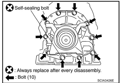
7. Tap rear extension assembly with soft hammer.
