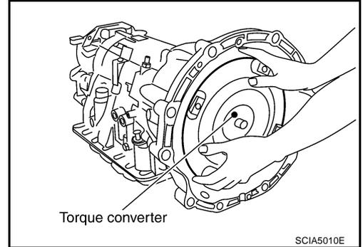
3. Check torque converter one-way clutch using check tool as shown at figure.
