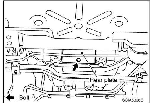
15. Turn crankshaft, and remove the four tightening bolts for drive plate and torque converter.
