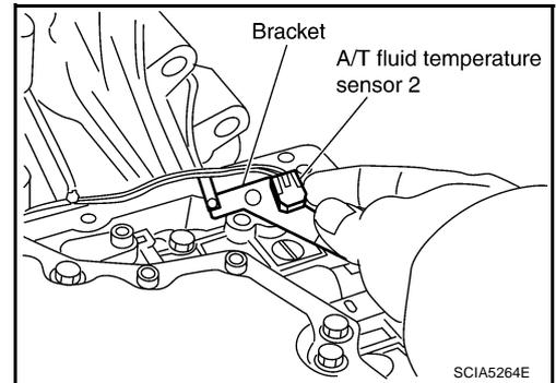
2. Install A/T fluid temperature sensor 2 (with bracket) in control valve with TCM.
