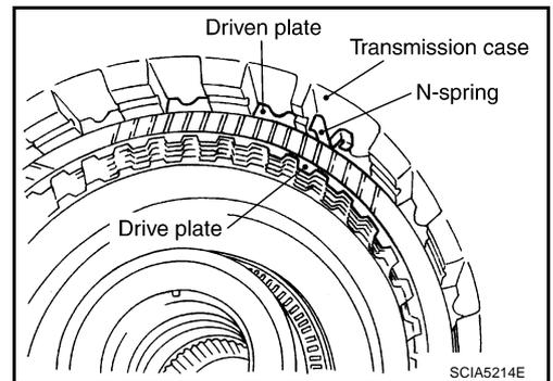
53. Remove reverse brake drive plates, driven plates and dish plate from transmission case.
