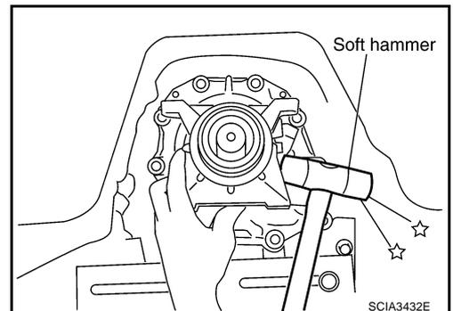
12. Remove rear extension assembly from transmission case. (With needle bearing.)
