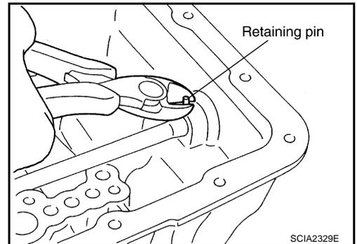
62. Remove manual plate (with parking rod) from manual shaft.
