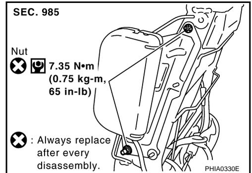
5. Remove front side air bag module fixing special nuts, then remove front side air bag module from bracket.
