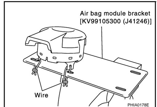
4. Connect deployment tool adapter (SST: J38381-80) to air bag module connector and deployment tool connector [SST: KV9910400 (J38381)].
