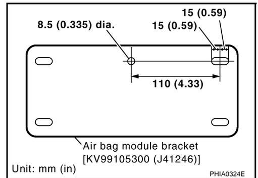
2. Firmly secure air bag module bracket [SST: KV99105300 (J41246)] with air bag module attached, in a vise.
