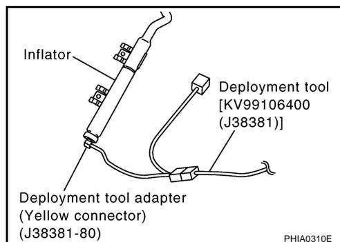
3. Put the inflator connected with the deployment tool [SST: KV99106400 (J38381)] into a tire without a wheel.
