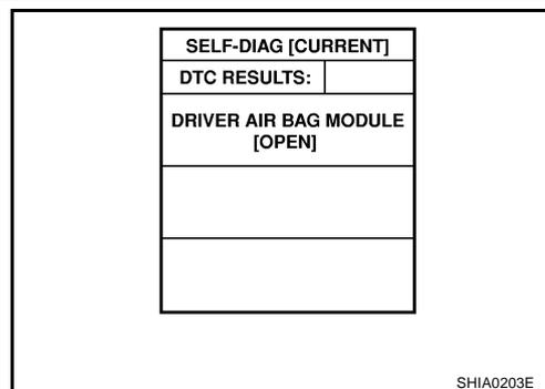
If no malfunction is detected on “SELF-DIAG [CURRENT]” even though malfunction is detected in “SRS Operation Check”, check the battery voltage. If the battery voltage is less than 9V, charge or replace the battery. Then go to [SRS-23. "DIAGNOSTIC PROCEDURE 3"](#) . If the battery voltage is OK, go to [SRS-25. "DIAGNOSTIC PROCEDURE 4 \(CONTINUED FROM DIAGNOSTIC PROCEDURE 2\)"](#) to diagnose the following cases:
