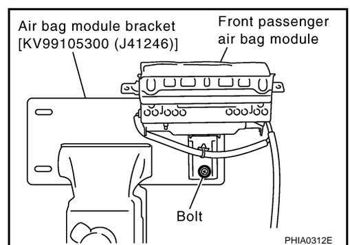
3. Connect deployment tool [SST: KV99106400 (J38381)] and deployment tool adapter (SST: J38381-65) to front passenger air bag module connector.
