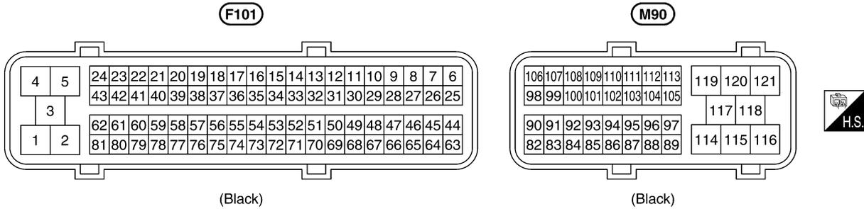
ABS ACTUATOR AND ELECTRIC UNIT (CONTROL UNIT)
