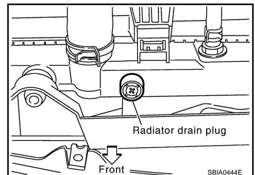
When drain all of engine coolant in the system, open water drain plugs on engine cylinder block. Refer to [EM-121, "DISASSEMBLY"](#).
