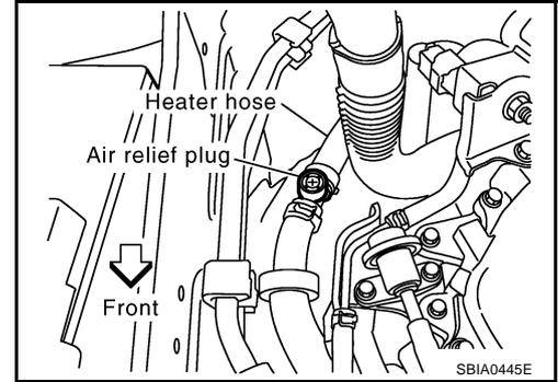
3. Fill radiator and reservoir tank to specified level.
