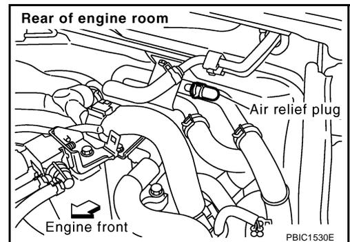
3. Fill thermostat housing and reservoir tank to specified level.
