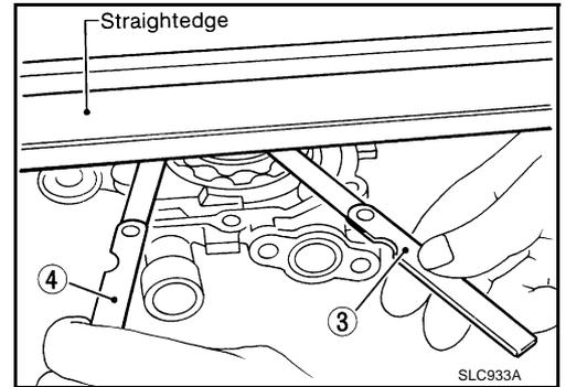
Calculate the clearance between oil pump inner rotor and oil pump body as follows.
