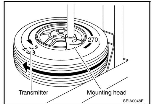
4. Lubricate tire well and fit second side of tire as normal. Ensure that tire does not rotate relative to rim.
