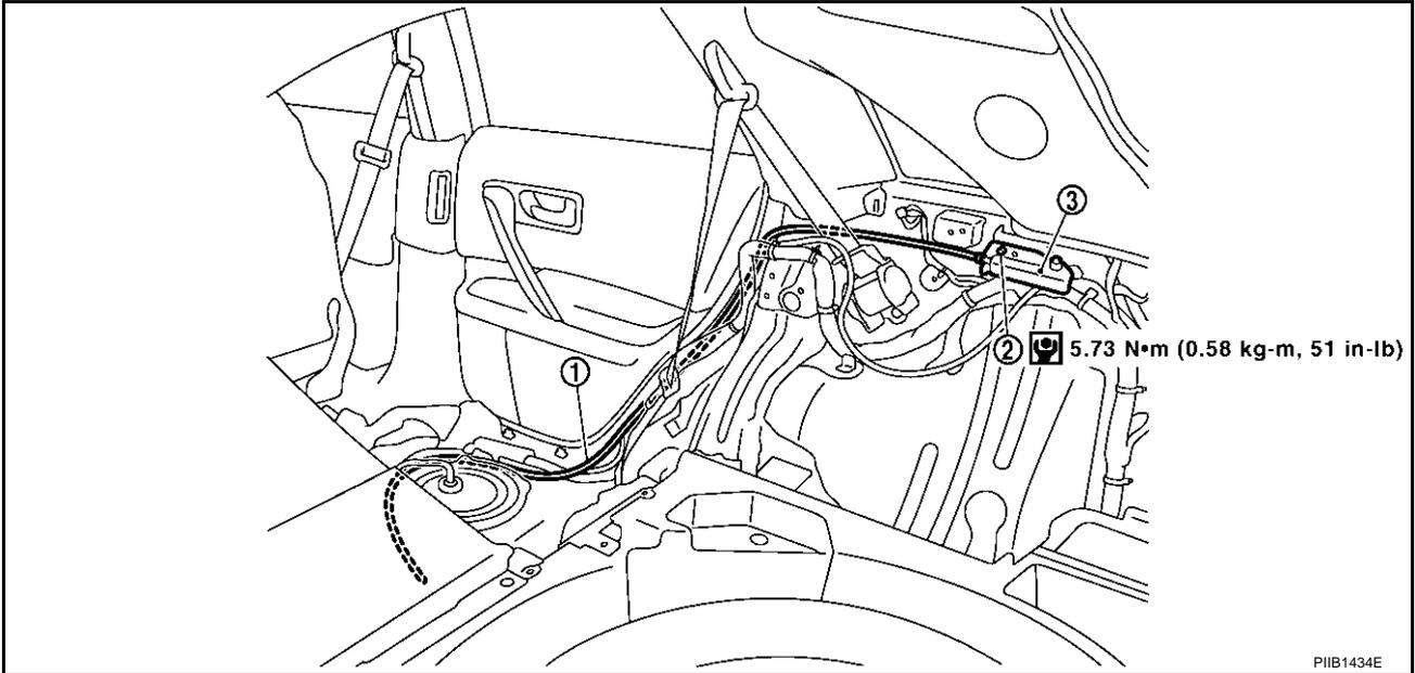
1. Remote control wire                      2. Bolt                                      3. Remote control lever
