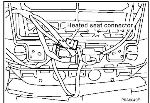
7. After removing the seatback trim and pad, remove the hog rings to separate the trim, pad, and seatback heater unit.
