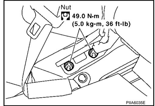
3. Remove the seatback mounting bolt and nut. Remove the remote control wire.
