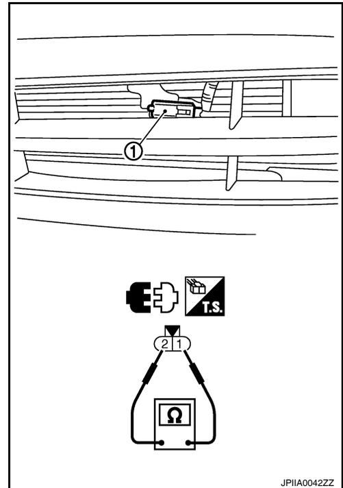
If NG, replace ambient sensor. Refer to [VTL-11. "Removal and Installation"](#).
