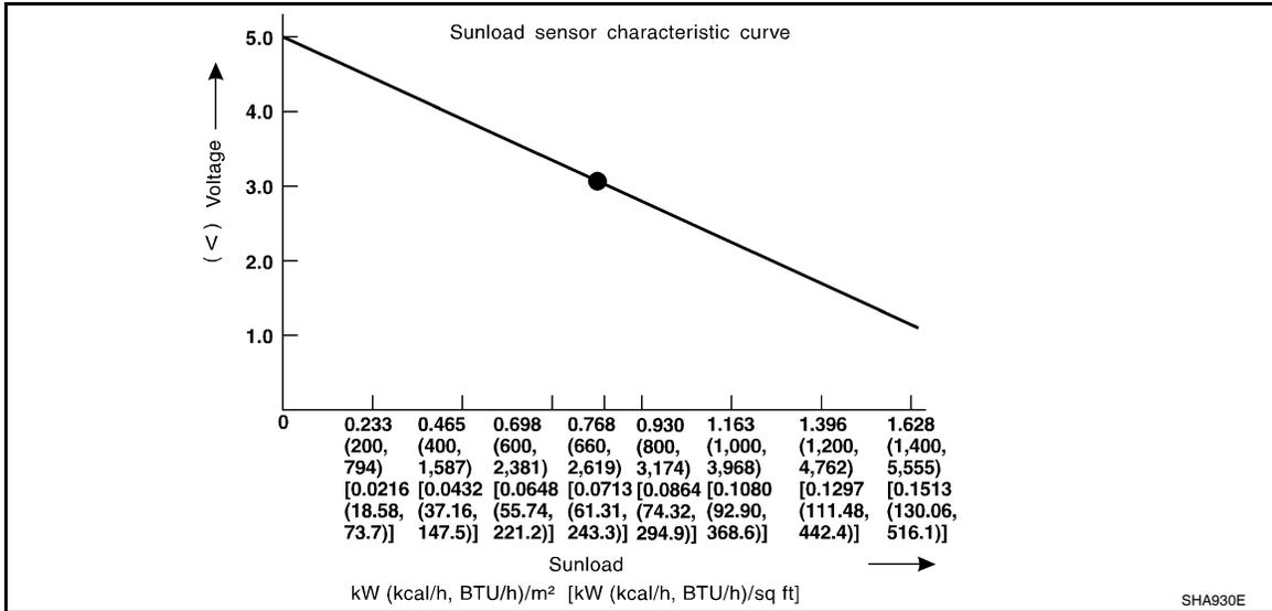
If NG, replace sunload sensor. Refer to [VTL-10, "Removal and Installation"](#).
