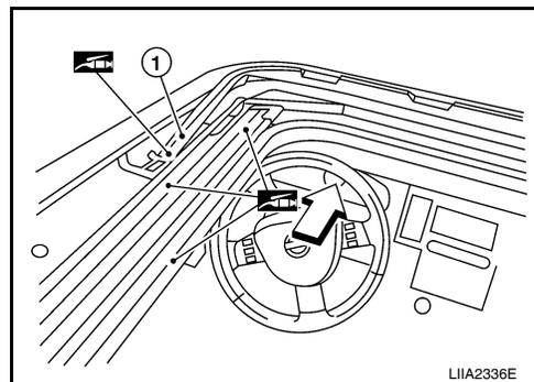
4. Check that the wind deflector (1) moves freely within the sunroof unit assembly while manually pressing down and releasing. If a malfunction is detected, remove the sunroof unit assembly and visually inspect; refer to [RF-91, "Inspection"](#). If damage is found, replace either wind deflector (1) or sunroof unit assembly as required.
