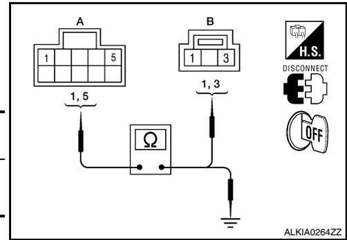
4. Check continuity between sunroof motor assembly connector (A) and ground.
