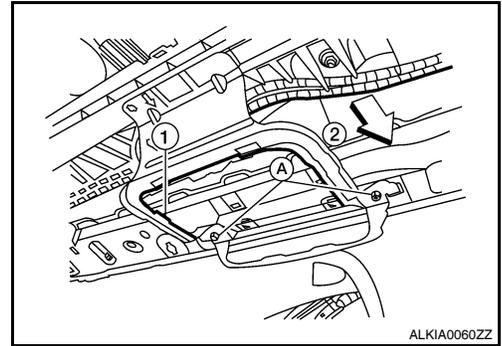
6. Remove bolts on the front end and side rails of the sunroof unit assembly.
