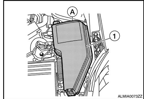
3. Disconnect the harness connectors from the IPDM E/R.
