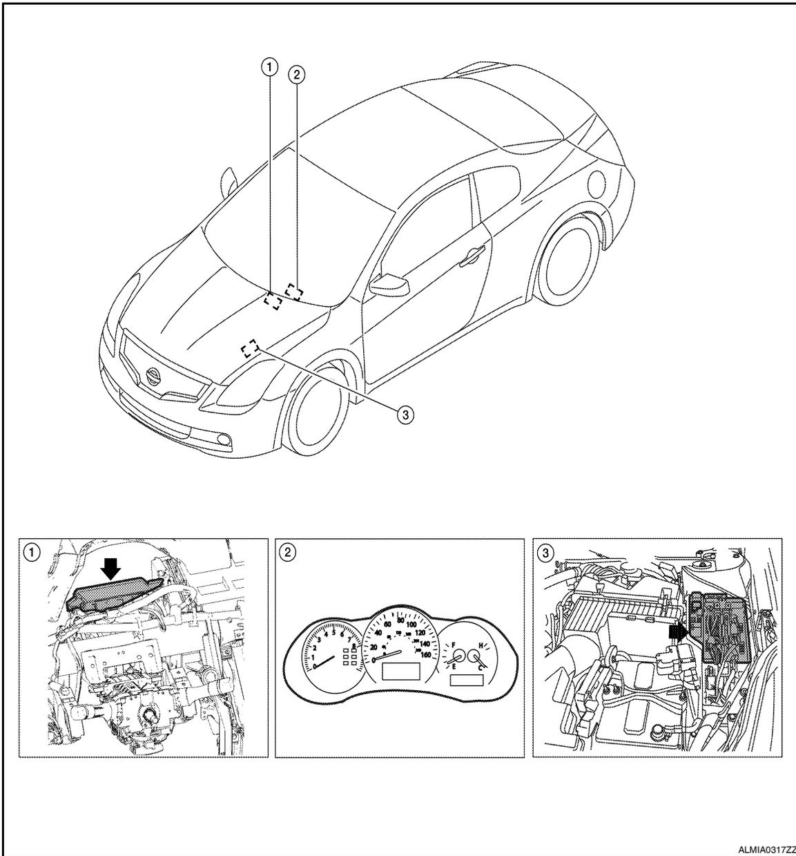
1. BCM M16, M17, M18, M19, M20, M21 (view with instrument panel removed)
