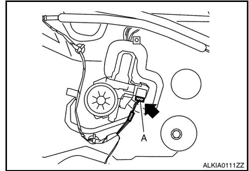
8. Remove the door module assembly.
