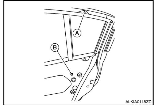
8. Remove the partition glass from the inside of the door in the direction as shown.
