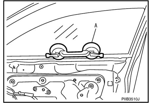
7. Disconnect the window motor connector (A).
